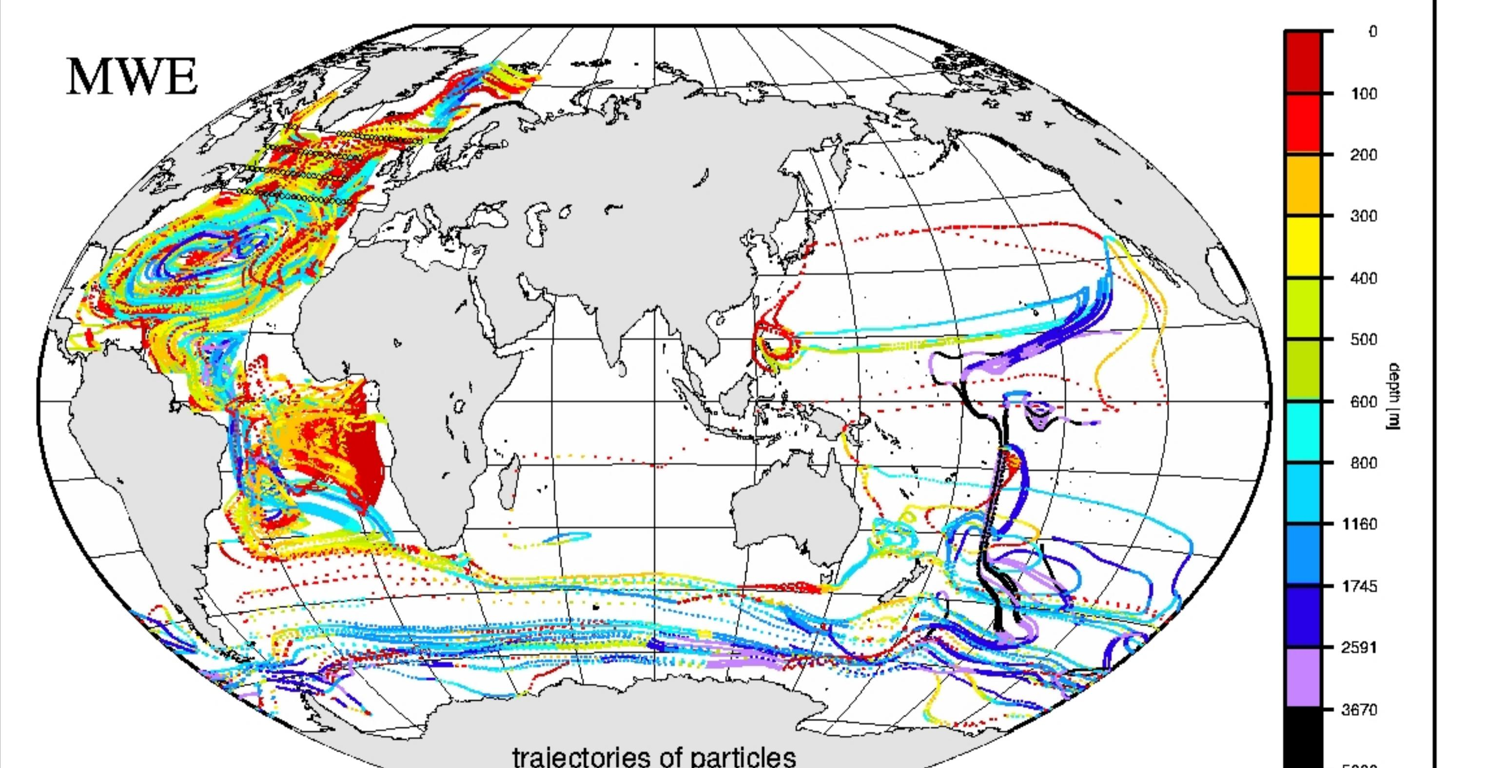
Trajectories of particles deployed in the northern North Atlantic. The depth is indicated by colors palette; as the particle descends or upwells the color of the trajectory changes.
