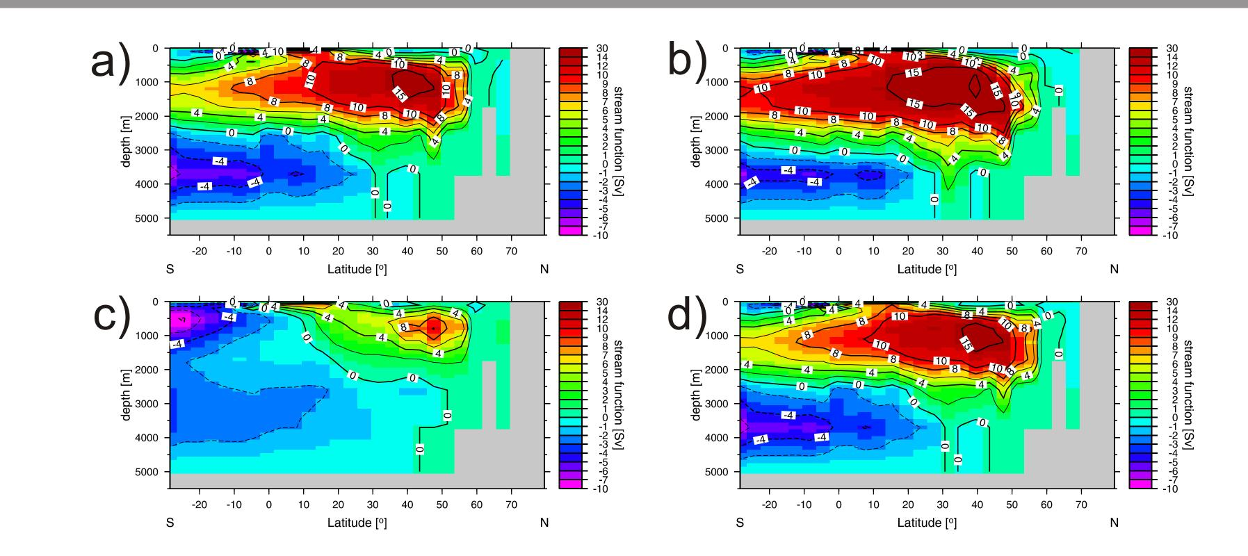
Figure 2. Meridional overturning in the Atlantic Ocean in the experiments shown in Table 1; (a) present-day; (b) Exp. 2; (c) Exp. 3; (d) Exp. 4. Streamfunction is shown in Sv (1 Sv =  $10^6$ m<sup>3</sup>/s). Areas with negative values are shaded.
