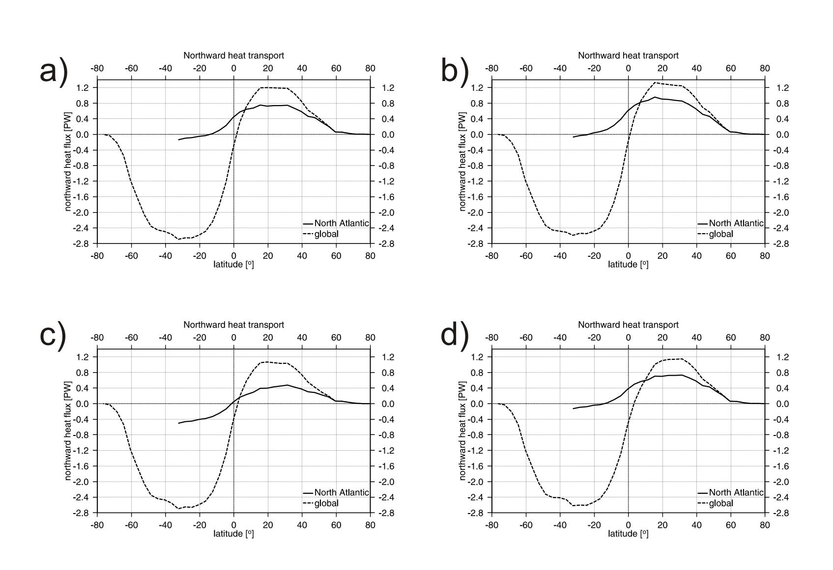
Figure 3. Northward heat transport (in PW; 1 PW = 10<sup>15</sup> W) in the Atlantic Ocean (solid line) and global (dotted line): (a) present-day; (b) Exp. 2; (c) Exp. 3; (d) Exp. 4; see Table 1.
