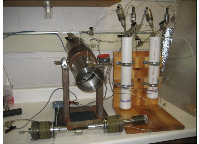
Fig. 1: Hydraulic fracturing system. Containment vessel with platen and fluid feed assembly and cell end-caps in foreground.
