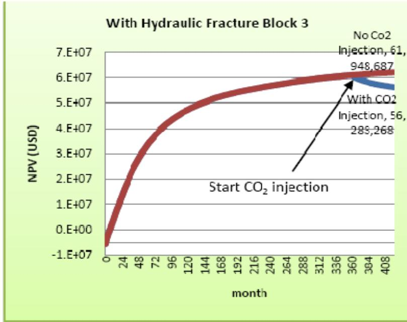
Figure 80: Comparison between with and without CO2 injection for block 3
