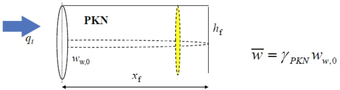
Figure 3: The PKN model describe fracture with a constant height.<sup>4</sup>
