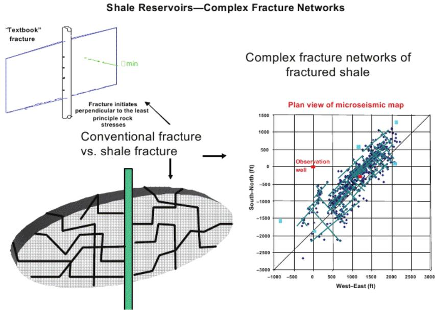
**Figure 1: Real fractures in shale reservoir vs equal main fracture<sup>1</sup>**
