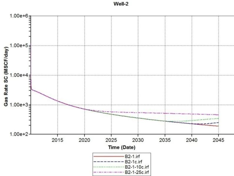
Figure 62: Methane Production Rate for different Injection Scenarios
