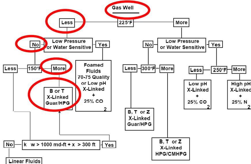
Figure 27: Fracture fluid selection chart<sup>14</sup>
