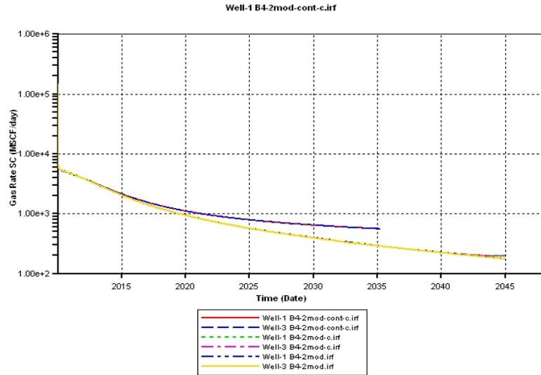
Figure 66: Production Rate for Block 4 Case 2 with early Continuous CO2 Injection
