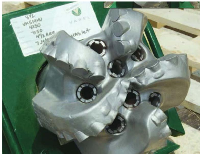
**Figure 24: A VM519HU drill bit designed by Varel International and Chesapeake Energy for drilling in the Barnett Shale. The new design, optimized for improved hydraulic flow and increased rate of penetration, has five blades, 3/4 in. cutters and a hydraulic package**
