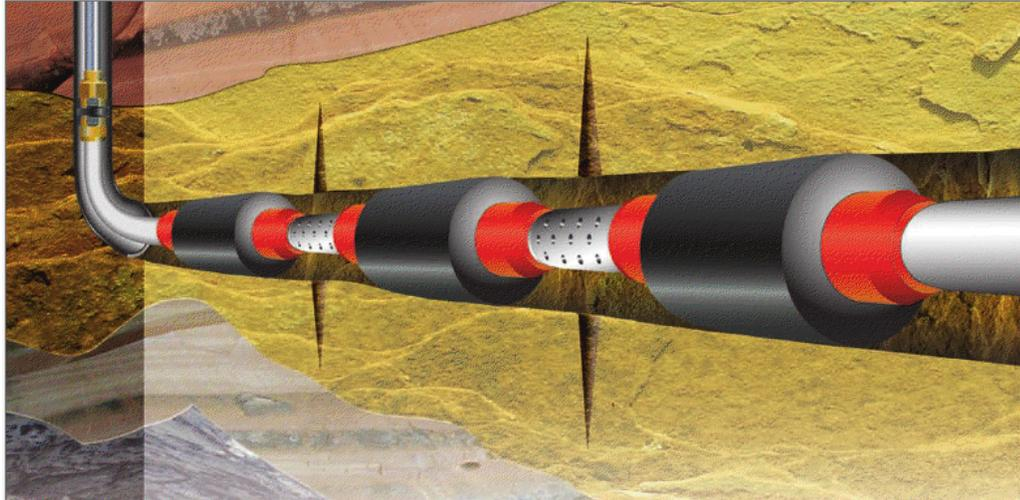
Figure 25: Horizontal well with multi fracture stages<sup>12</sup>
