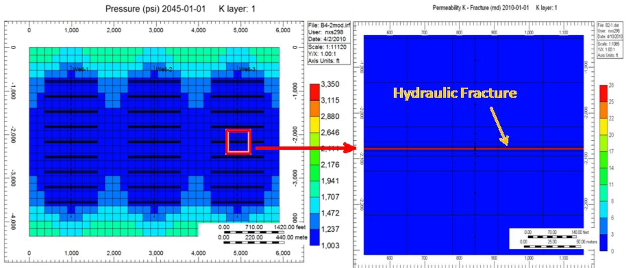
Figure 32: Local Grid Refinements to Model Hydraulic Fracture
