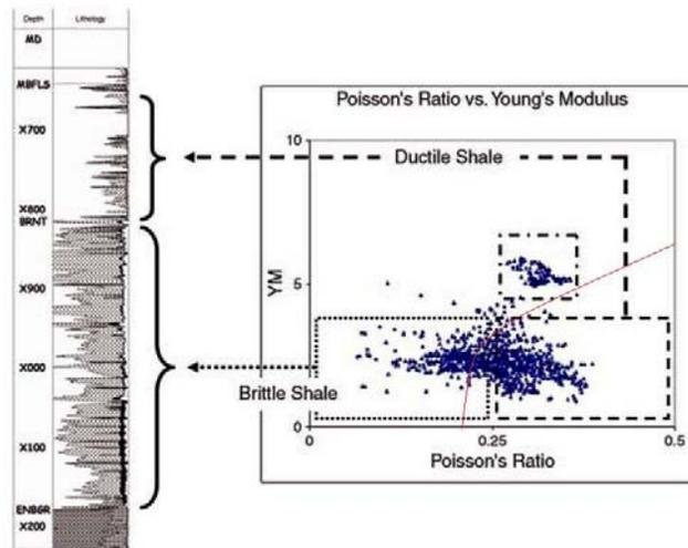
Figure 15: North Texas Barnett log strip showing brittle/ductile shale intervals from Young's modulus and Poisson's ratio cross-plot. (Source: Grieser and Bray; Identification of Production Potential in Unconventional Reservoir, 2007)
