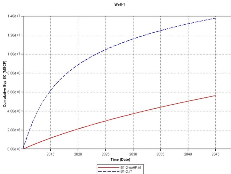
**Figure 35: Cumulative production comparisons between well with hydraulic fracture and without hydraulic fracture**
