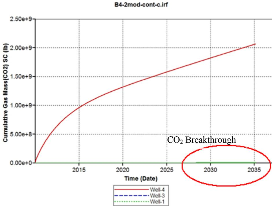
Figure 68: CO2 Injection for Block 4 Case 2 with early continuous CO2 Injection
