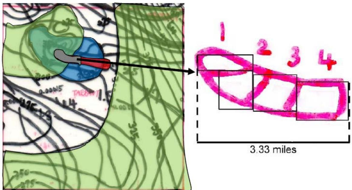
Figure 22: Divide reservoir into four homogeneous blocks
