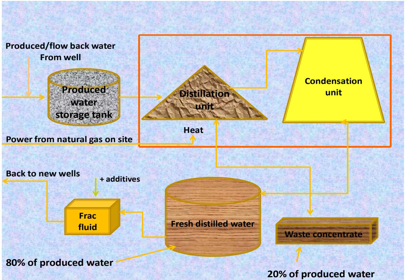
Figure 36: Schematic Diagram of our Recycling Technique
