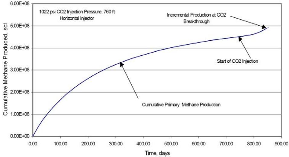
**Figure 10: Incremental methane produced by CO<sub>2</sub> injection after primary depletion<sup>11</sup>**
