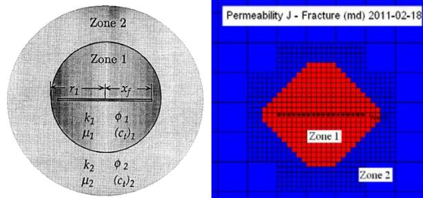
Figure 7: Composite Model of Naturally Fractured Reservoir<sup>7</sup>
