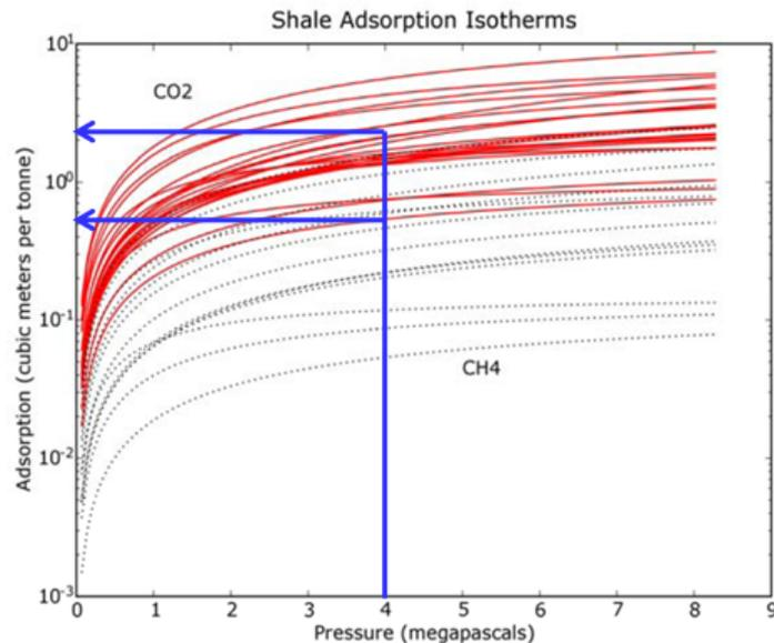
Figure 9: CH<sub>4</sub> and CO<sub>2</sub> Isotherm for Shale (Nuttall et al., 2006)
