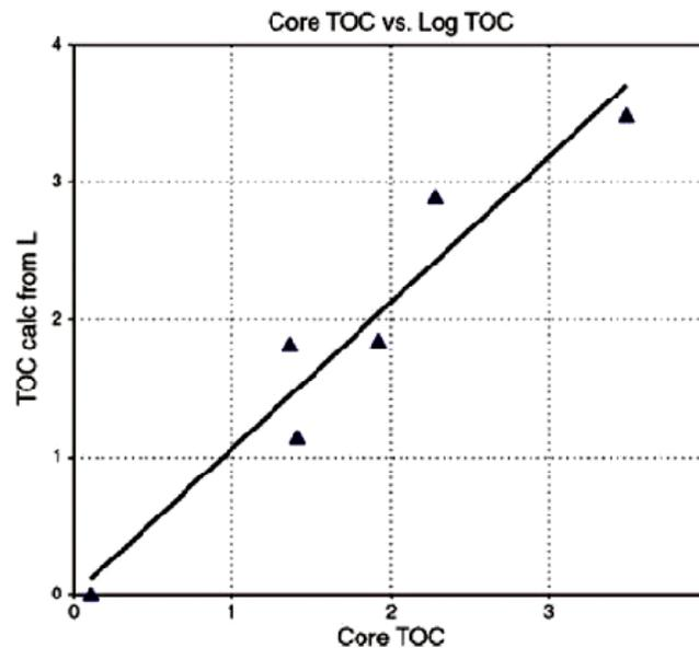
Figure 13: Comparison of core-derived TOC with estimated TOC from resistivity/porosity log data.(Source: Grieser and Bray; Identification of Production Potential in Unconventional Reservoir,2007)
