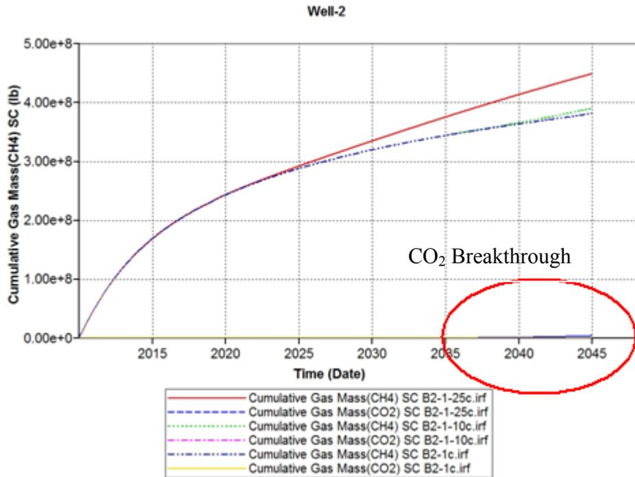
Figure 65: Methane and CO<sub>2</sub> Production
