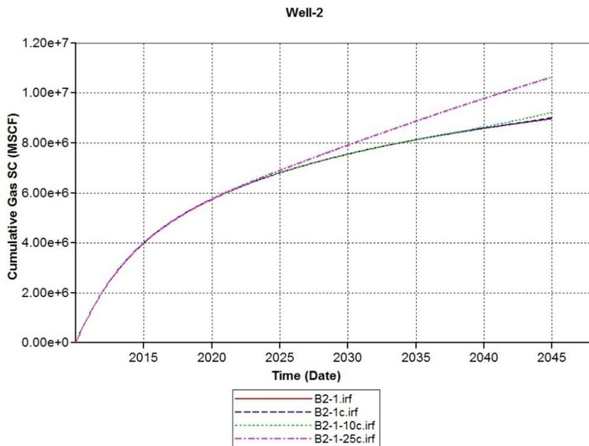
Figure 63: Cumulative Gas Production for different Injection Scenarios
