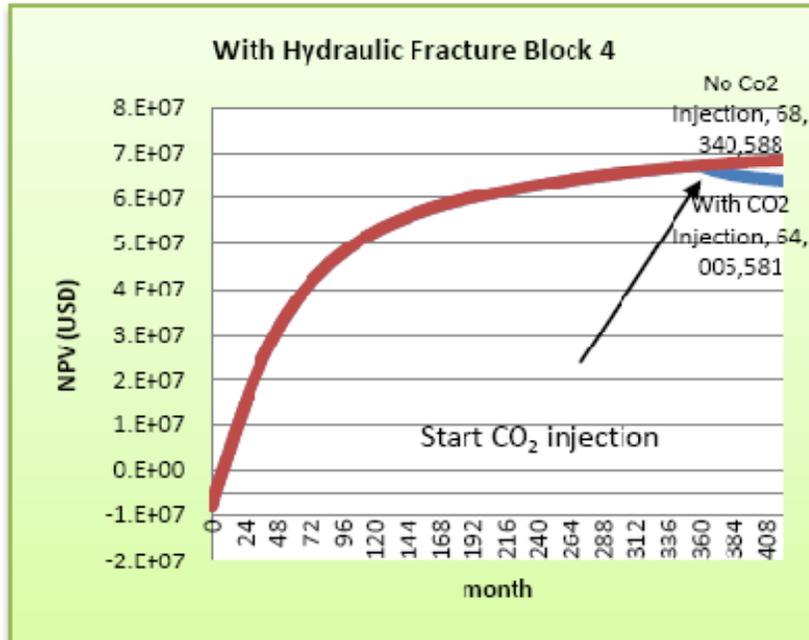
Figure 81: Comparison between with and without CO2 injection for block 4
