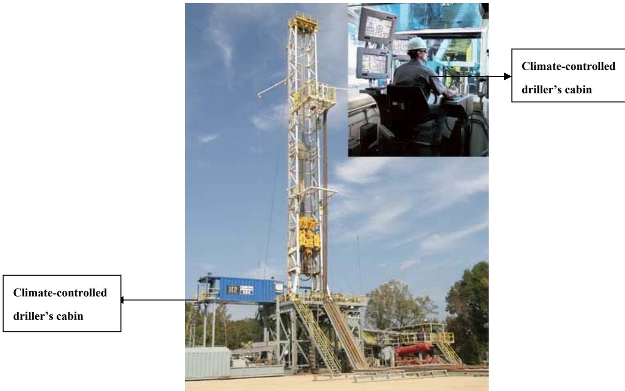
**Figure 23: A Flex Rig, and a Climate-controlled driller's cabin on the latest generation Flex Rig allowed addition of more electronic controls, and joystick controls for block**
