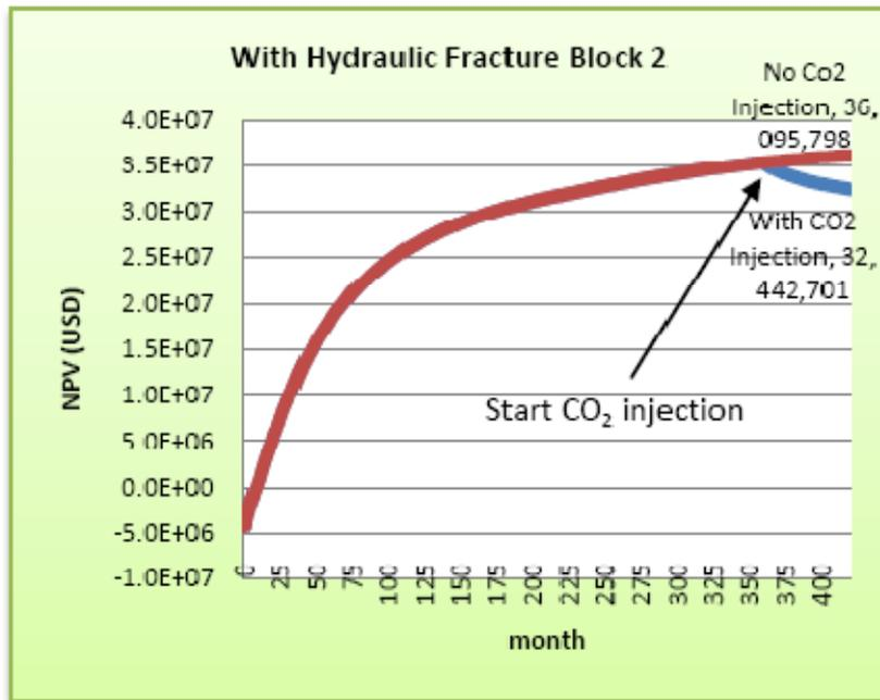
Figure 79: Comparison between with and without CO<sub>2</sub> injection for block 2
