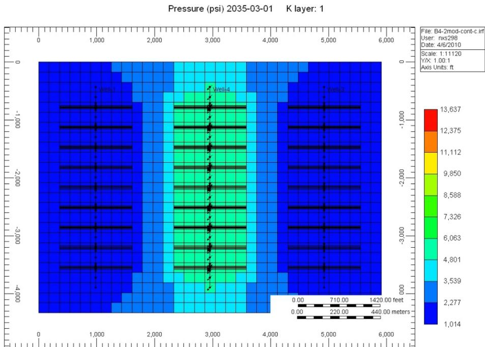
Figure 69: Pressure distribution after 25 years for Block 4 Case 2 with early CO2 Injection
