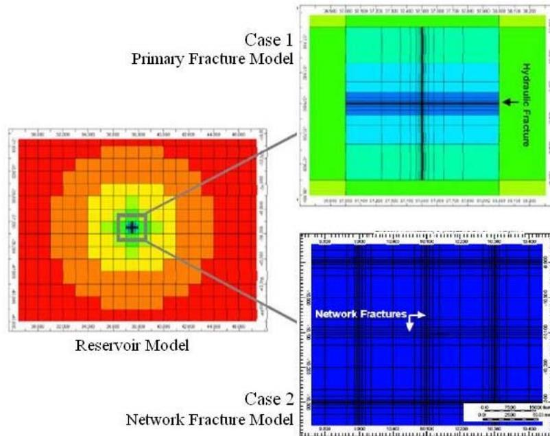
Figure 8: Primary Fracture Model and Network Fracture Model from CMG<sup>8</sup>
