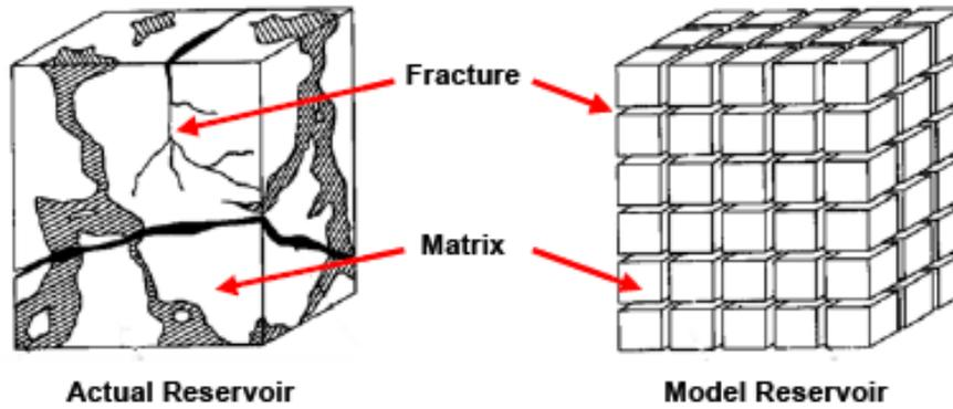
Figure 6: Actual and idealized model of natural fracture<sup>6</sup>
