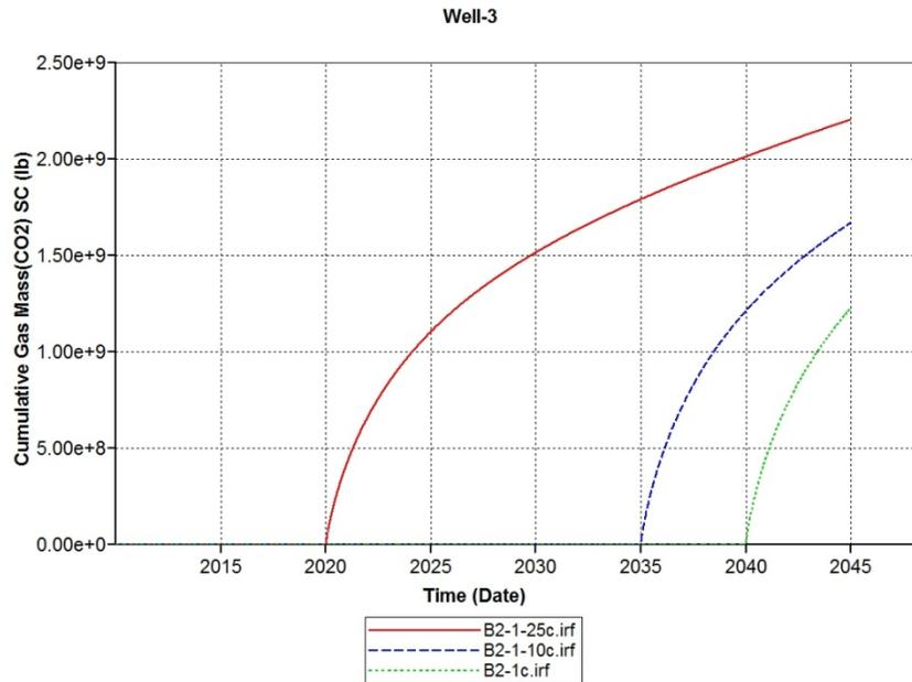
**Figure 64: Cumulative CO2 Injection for different Injection Scenarios**
