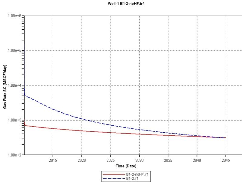
**Figure 34: Production rate comparisons between well with hydraulic fracture and without hydraulic fracture**
