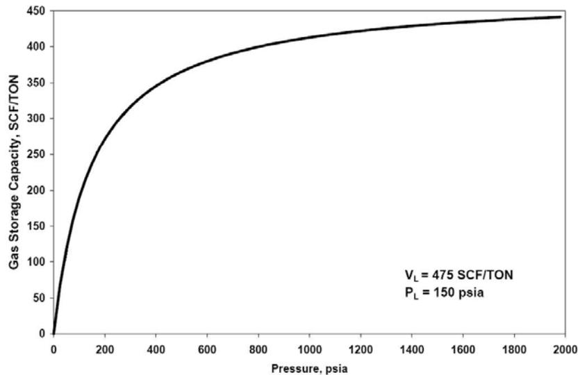
**Figure 5: Langmuir Isotherm<sup>5</sup>**
