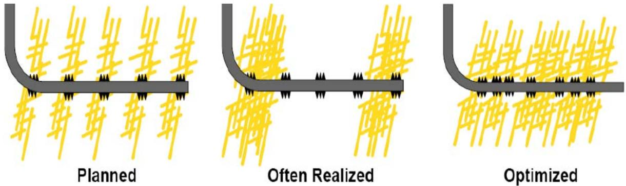
**Figure 2: fracture distribution on the horizontal well<sup>2</sup>**
