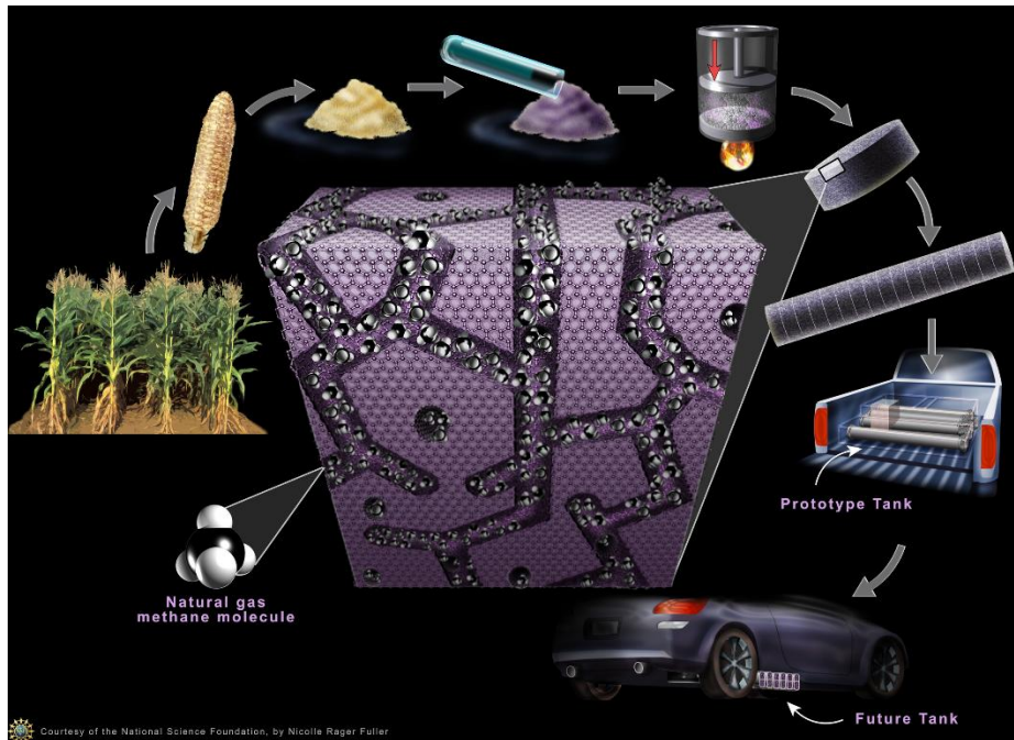
Figure 32. Development of Nanoporous Carbon Material from Corncob waste to Store Methane.
