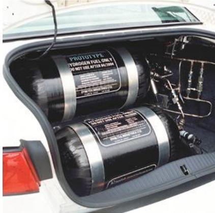
Figure 36: Ford hydrogen I.C.E. prototype storage cells
