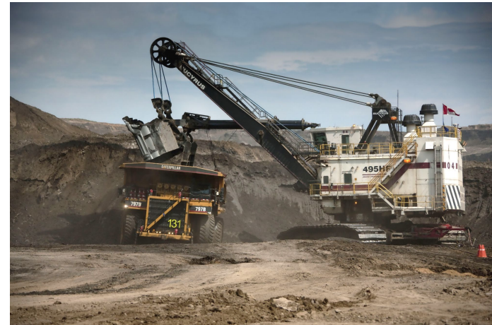
A rope shovel and CAT 797 400 ton haul truck in the oil sands
