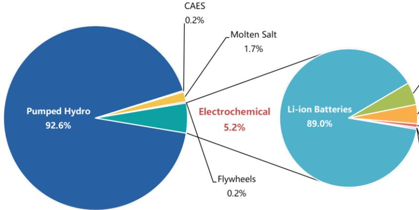
► Pumped storage hydropower is the world's largest battery technology,
