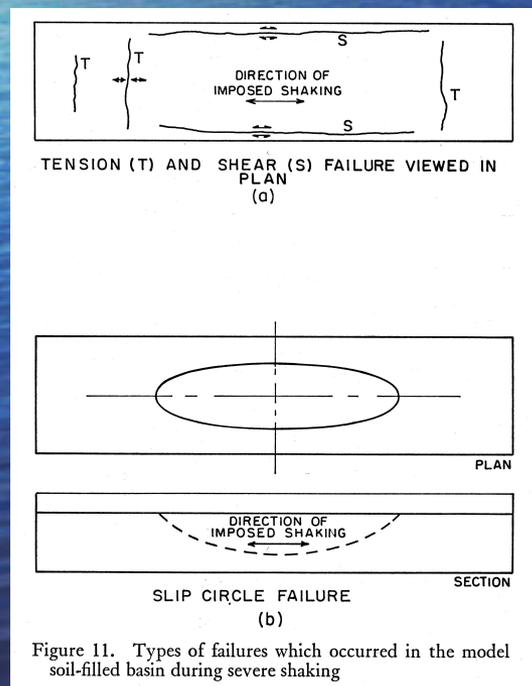
Figure 11. Types of failures which occurred in the model soil-filled basin during severe shaking
