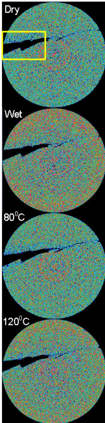
**Figure 3.** Scanning sequences for the core 57 mm downstream of the inlet of the 90 mm long core. Scans are for the initial dry core, and then wet at 20°C, 80°C and 120°C. The boxed region is processed in Figure 4 to define dissolved mass and relative displacement of fracture faces.
