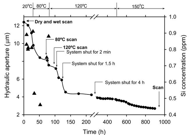
**Figure 2.** Change in fracture aperture with test duration. Hydraulic aperture evaluated from measured steady flux and axial pressure differential (equation (1)). Scan sequences, temperature transitions, brief test interruptions and aqueous concentrations of silicon measured from the effluent fluid (triangles) are noted.
