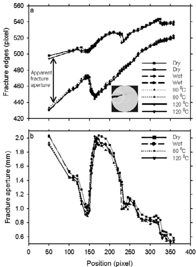
**Figure 4.** Distribution of fracture aperture, evaluated across the observed fracture 57 mm downstream of the inlet. Profiles are shown for (a) positions of the fracture walls, and for (b) fracture aperture. Data reduced for scans completed dry, and wet at 20°C, 80°C and 120°C.
