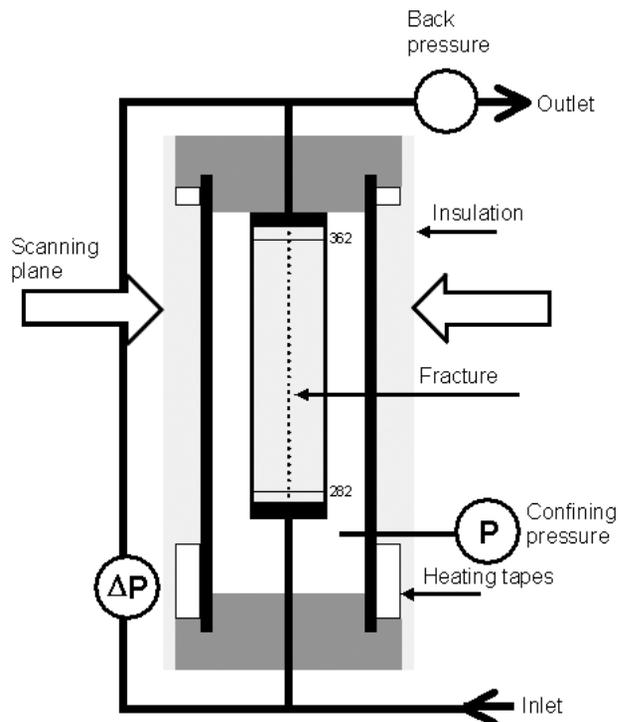
**Figure 1.** Schematic of flow-through experiment. Pre-heated water is circulated through the uniformly heated interior core sample and effluent pipe.
