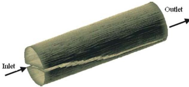
**Fig. 1** Schematic representation of the fractured core used in X-Ray CT experiments
