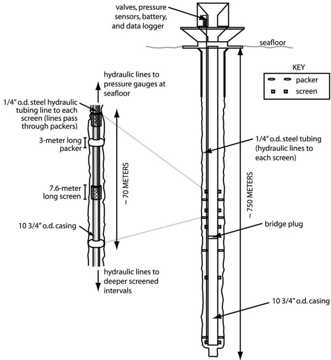
**Figure 8.** ACORK design at ODP Site 1173. (left) Detailed view of packers and screens. Horizontal exaggeration is approximately 20:1 (screen height is actually 25 times the screen radius). (right) Hydraulic tubing connects screens with pressure sensors at the seafloor. The bridge plug at ODP Site 1173 set prematurely during installation at  $\sim 466$  m below seafloor (mbsf).
