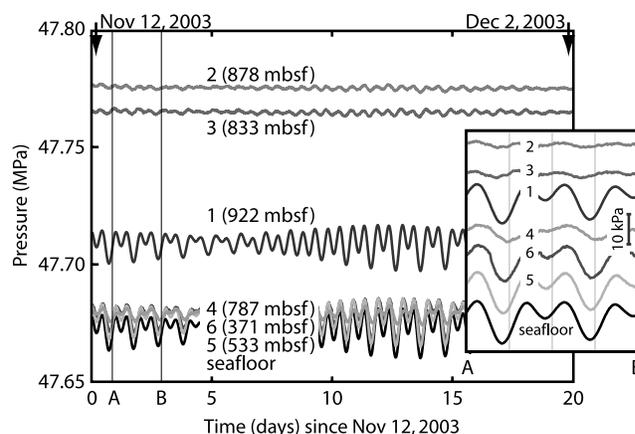
**Figure 10.** Typical pressure record at ODP Site 808. Pressure is slightly elevated above hydrostatic ( $<0.2$  MPa) at screens 2 and 3. Inset shows mean-removed pressures over the 2-day window A–B. Screens 2, 3, and 4 have visibly diminished amplitudes and large phase shifts.
