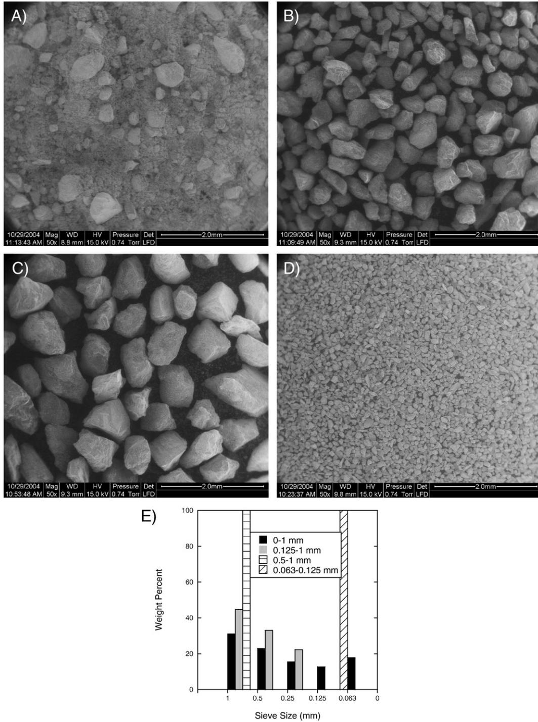
Fig. 5. Grain-size distributions of materials recovered from Soufrière Hills volcano. SEM photos (A–D) are all at 50× magnification with a scale bar length of 2 mm. (A) All material passing a 1 mm sieve. (B) All material coarser than 0.125 mm and finer than 1 mm. (C) Material finer than 1 mm and coarser than 0.5 mm. (D) Material finer than 0.125 mm and coarser than 0.063 mm. (E) Histogram showing the abundance of grain-size ranges in experimental samples.
