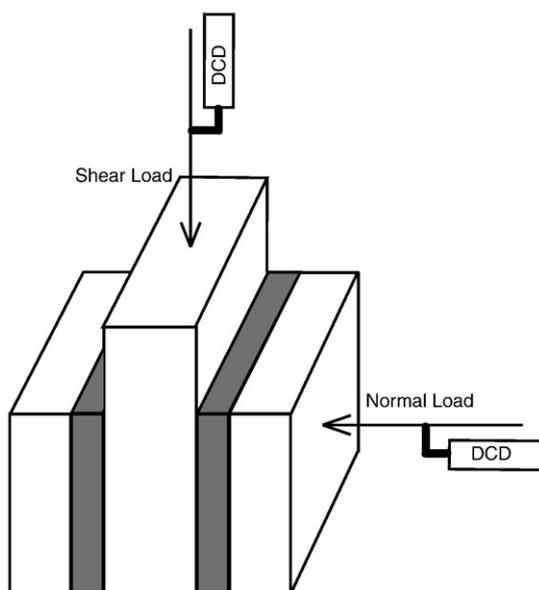
Fig. 3. Schematic illustration of the double-direct shear friction configuration showing the orientation of the sample set-up and the direction of applied normal and shear stresses.
