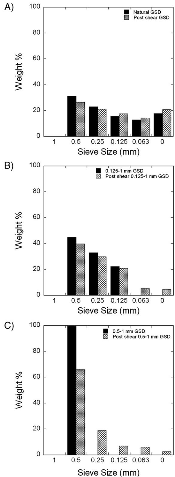
Fig. 9. Grain-size distribution of the natural SHV sample (< 1 mm) shown before and after shearing. Experiments shown were run at 0.75 MPa normal stress and at a shear rate of 10 μm/s. (A) Experiment p521 with natural grain-size distribution. (B) Experiment p517 with initial grain-size distribution of 0.125–1 mm. (C) Experiment p507 with initial grain-size distribution of 0.5–1 mm.
