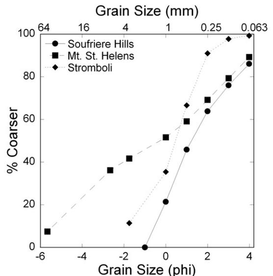
Fig. 2. Grain-size distributions for the materials tested. The Soufrière Hills pyroclastic flow material was sieved at 2 mm in the field and therefore the distribution curve is truncated at 2 mm. The grain-size distributions of the Mount St. Helens lahar and Stromboli pyroclastic flow materials are not truncated. Note that the Mount St. Helens and Soufriere Hills materials do not reach 100% because the grain-size scale does not go to zero.
