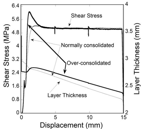
Fig. 12. Evolution of shear stress and layer thickness as a function of displacement for a sample of the natural grain-size distribution (<1 mm) of Mount St. Helens lahar. The results contrast response for a sample “normally consolidated” at a normal stress of 8 MPa (p567) and sheared at 10 μm/s (thin black line) with the same material pre-loaded to ~50 MPa (p566), then also sheared at a rate of 10 μm/s under a normal stress of 8 MPa (thick black line).
