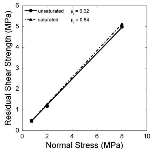
Fig. 7. Coulomb failure envelopes describing the failure criteria for a natural grain-size distribution (all materials  $< 1$  mm) of Soufrière Hills pyroclastic flow material in both saturated and unsaturated states. Tests were conducted at a shear rate of 10  $\mu\text{m/s}$  and at normal stresses of 0.75, 2, and 8 MPa.
