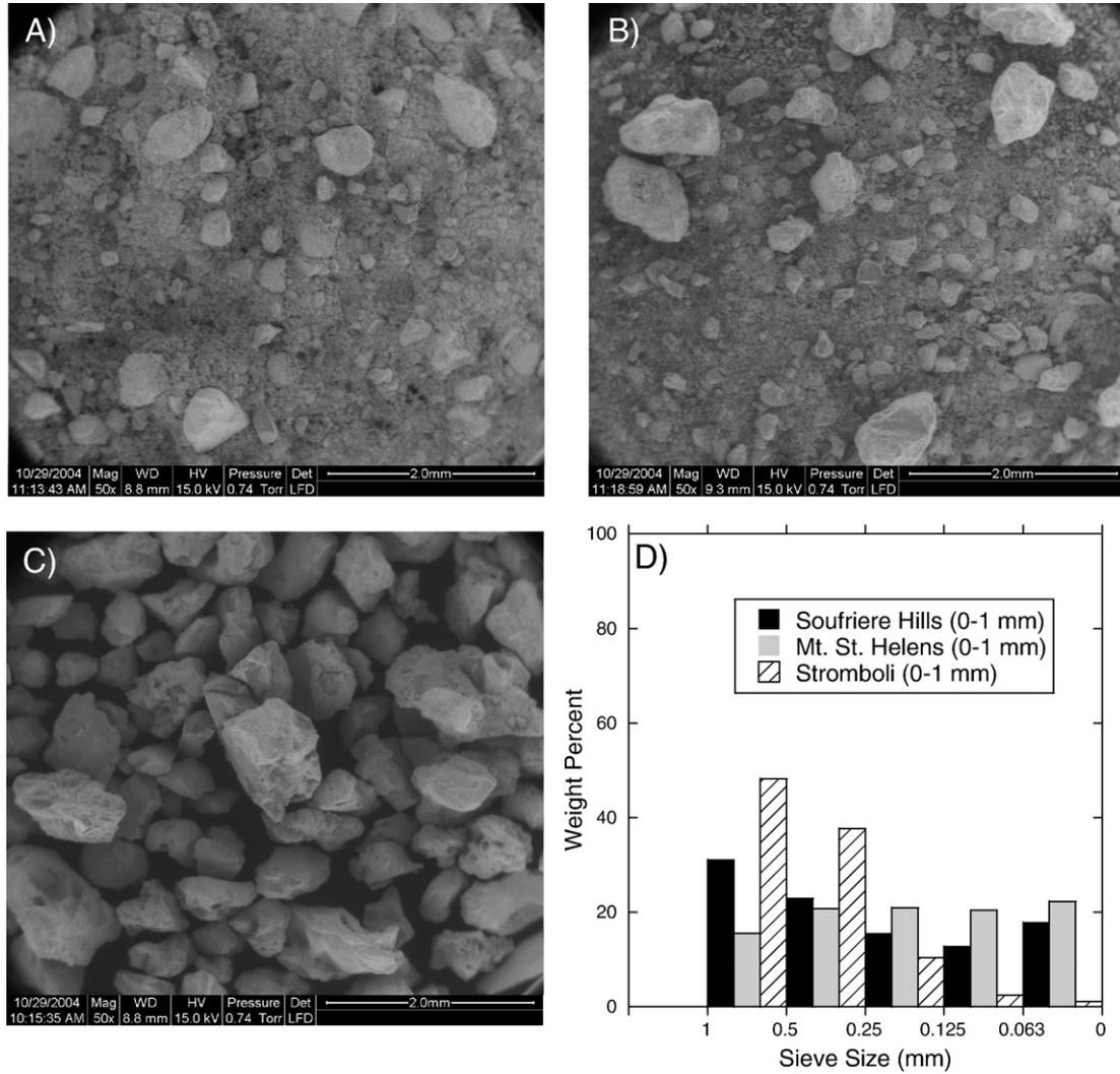
Fig. 10. Grain-size distributions of materials from Soufrière Hills, Stromboli, and Mount St. Helens. SEM photos (A–C) are all at 50× magnification with a scale bar length of 2 mm. All materials are the natural size distribution that passed a 1 mm sieve. (A) Soufrière Hills pyroclastic material (B) Mount St. Helens’s lahar material (C) Stromboli pyroclastic material (D) Histogram plot of the grain-size distribution of the materials.
