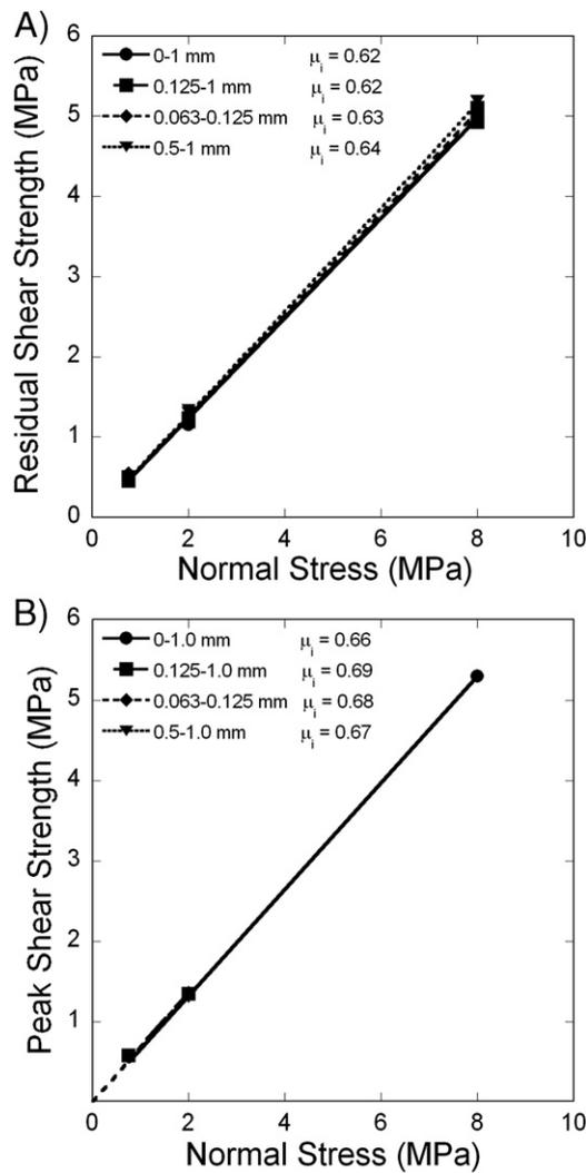
Fig. 6. Coulomb failure envelopes for the four different grain-size ranges of Soufrière Hills pyroclastic material. (A) Envelopes produced using residual shear strength. (B) Envelopes produced using available peak strength data. Tests were conducted at a shear rate of 10  $\mu\text{m/s}$  and at normal stresses of 0.75, 2, and 8 MPa. Note that in both panels several data points lie over one another. See Table 1 for complete data set.
