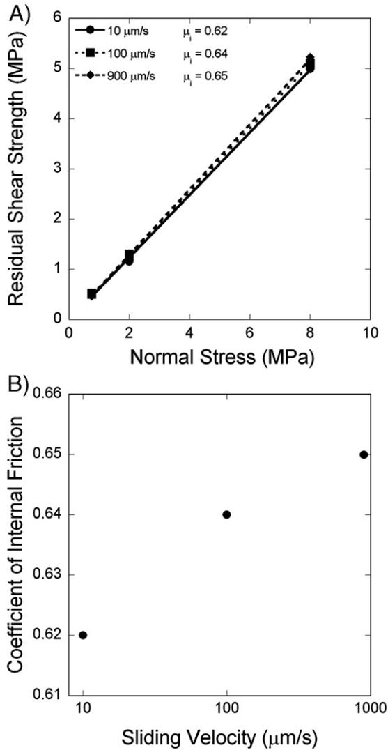
Fig. 8. (A) Coulomb failure envelopes for a natural grain-size distribution (all materials < 1 mm) of Soufrière Hills material for shear velocities of 10, 100, and 900 μm/s. (B) The sliding frictional strength of the layer is shown to increase with an increasing sliding velocity.
