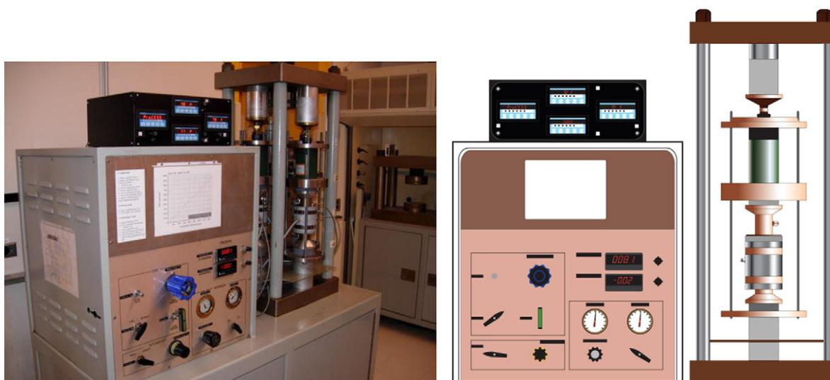
**Fig. 6.** Quadcell experimental arrangement showing four-part compression cell to apply constant stress to the top of a cylindrical sample of proppant sandwiched between wafers of host rock stagnant flow conditions.
