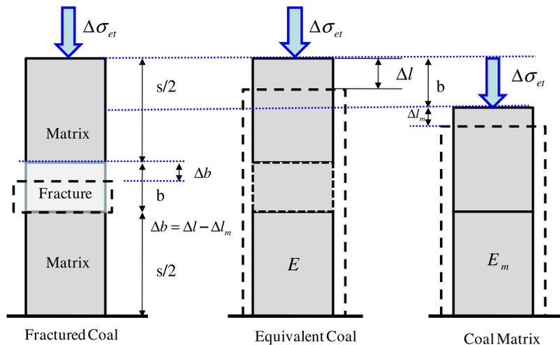
Fig. 12. Schematic diagram of fracture aperture interaction with effective stress.
