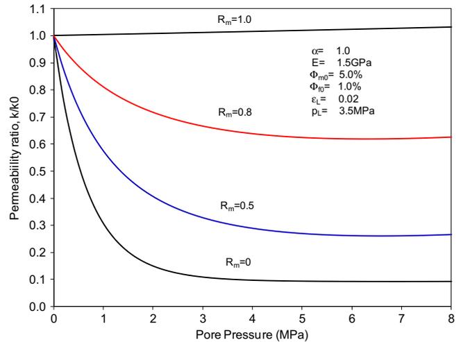
Fig. 13. Impact of partition coefficient on permeability change.
