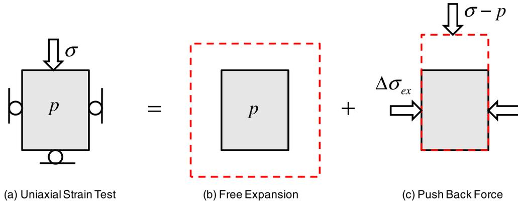
Fig. 2. Swelling tests under the uniaxial strain condition: (a) uniaxial strain condition; (b) free expansion due to gas sorption; (c) push back to original position by the resulting effective stress.
