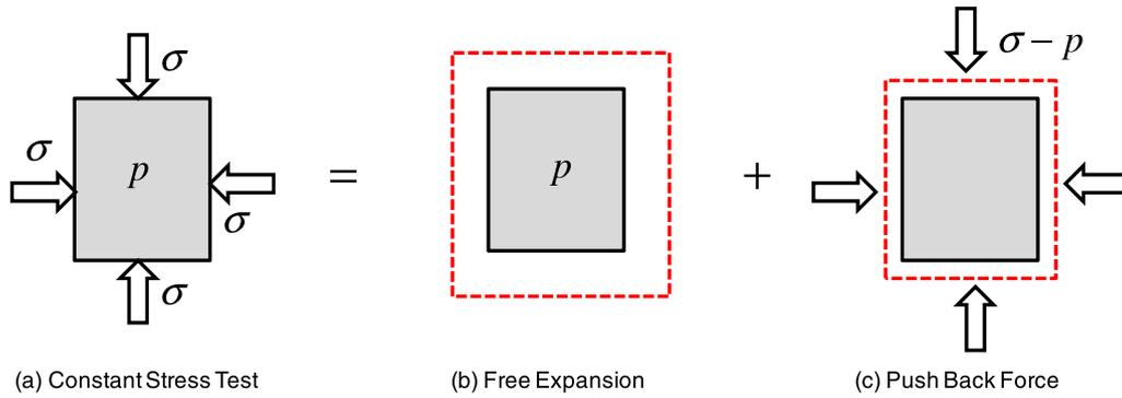
Fig. 9. Swelling tests under the stress controlled condition: (a) stress controlled condition; (b) free expansion due to gas sorption; (c) push back by the applied effective stress.
