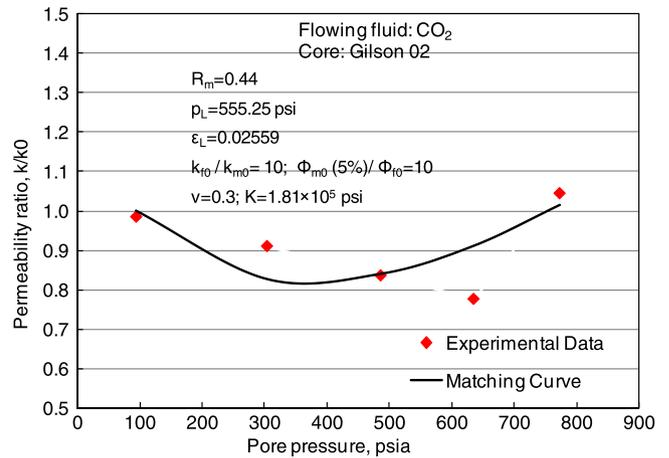
(c) Experimental data match for CO<sub>2</sub> for core Gilson 02.
