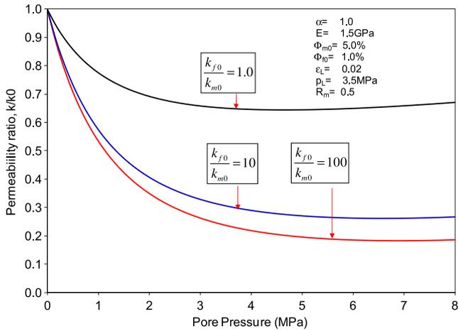
Fig. 14. Impact of the fracture permeability to matrix permeability ratio on permeability change.
