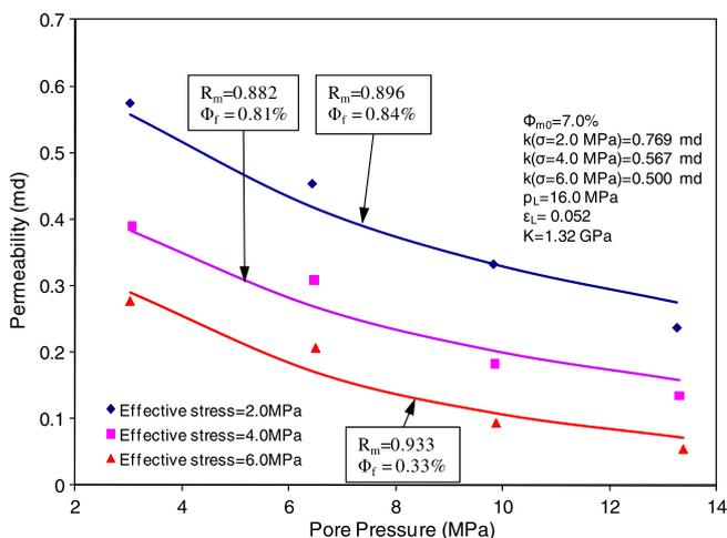
Fig. 16. Experimental data matching for constant effective stress case with  $\text{CO}_2$  injection.
