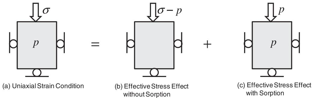
Fig. 3. Swelling tests under the uniaxial strain condition: (a) uniaxial strain condition; (b) effective stress effect without gas sorption; (c) effective stress effect with constrained gas sorption.
