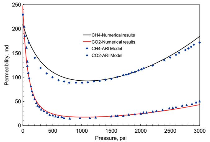
**Fig. 4.** Comparison with ARI model for CO<sub>2</sub> injection into a well in the San Juan Basin.
