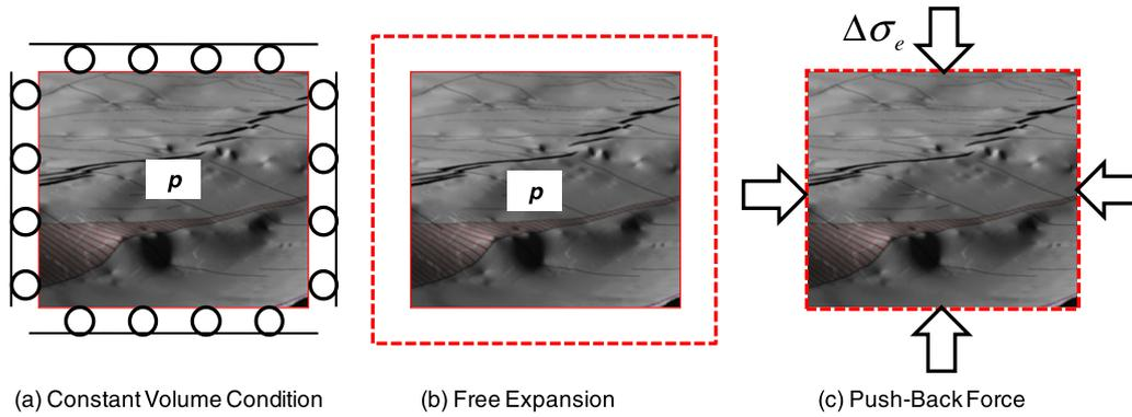
Fig. 6. Swelling tests under the constant volume condition: (a) constant volume condition; (b) free expansion due to gas sorption; (c) push back to original positions by the resulting effective stress.
