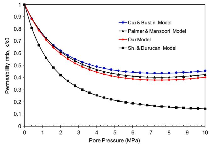
**Fig. 5.** Comparison between the proposed permeability model and three alternate models.
