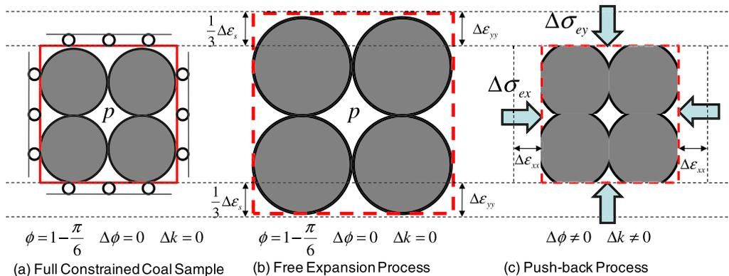
Fig. 1. Illustration of effective stress induced volume strain on permeability change.
