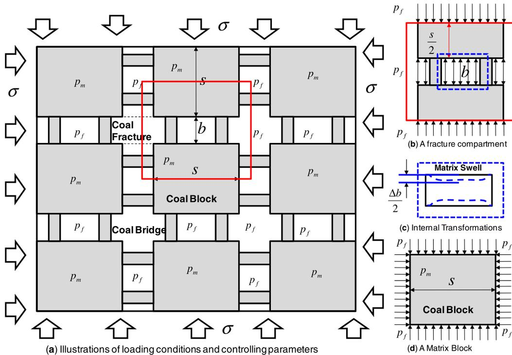
Fig. 11. Conceptual model for coal-matrix bridges.
