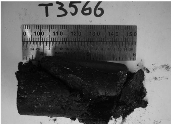
**Fig. 2.** Photograph of a fractured sample with a through-going shear fracture representing the failure mode.
