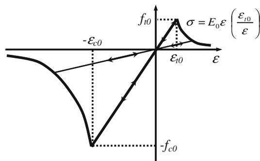
**Fig. 1** The elastic damage-based constitutive law of elements under uniaxial stress condition ( $f_{t_0}$  and  $f_{c_0}$  are uniaxial tensile strength and uniaxial compressive strength, respectively)
