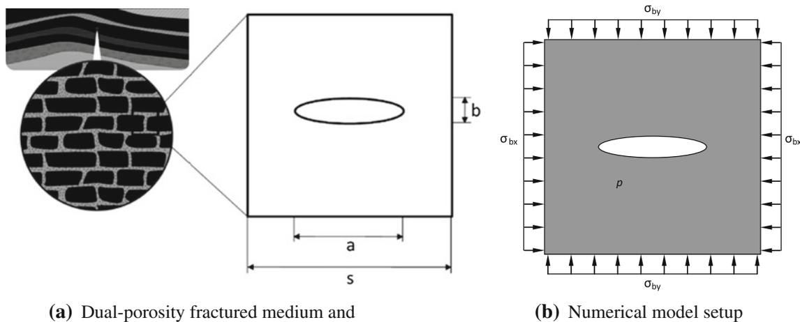
Fig. 2 Diagram for a dual-porosity fractured medium and b numerical model setup (Izadi et al. 2011)
