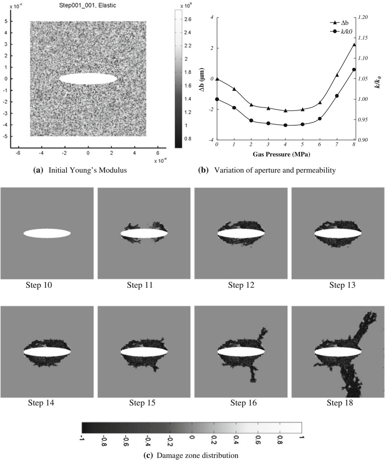
**Fig. 5** Numerical results for Scenario III: **a** initial Young's modulus, **b** variation of aperture and permeability with gas pressure, and **c** damage zone distribution
