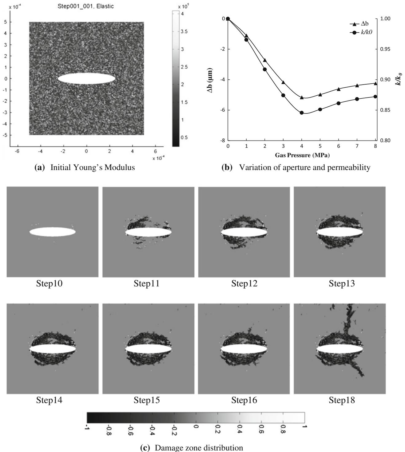
**Fig. 8** Numerical results for Scenario VI: **a** initial Young's modulus, **b** variation of aperture and permeability with gas pressure and **c** damage zone distribution for a homogeneity index  $m = 3.0$
