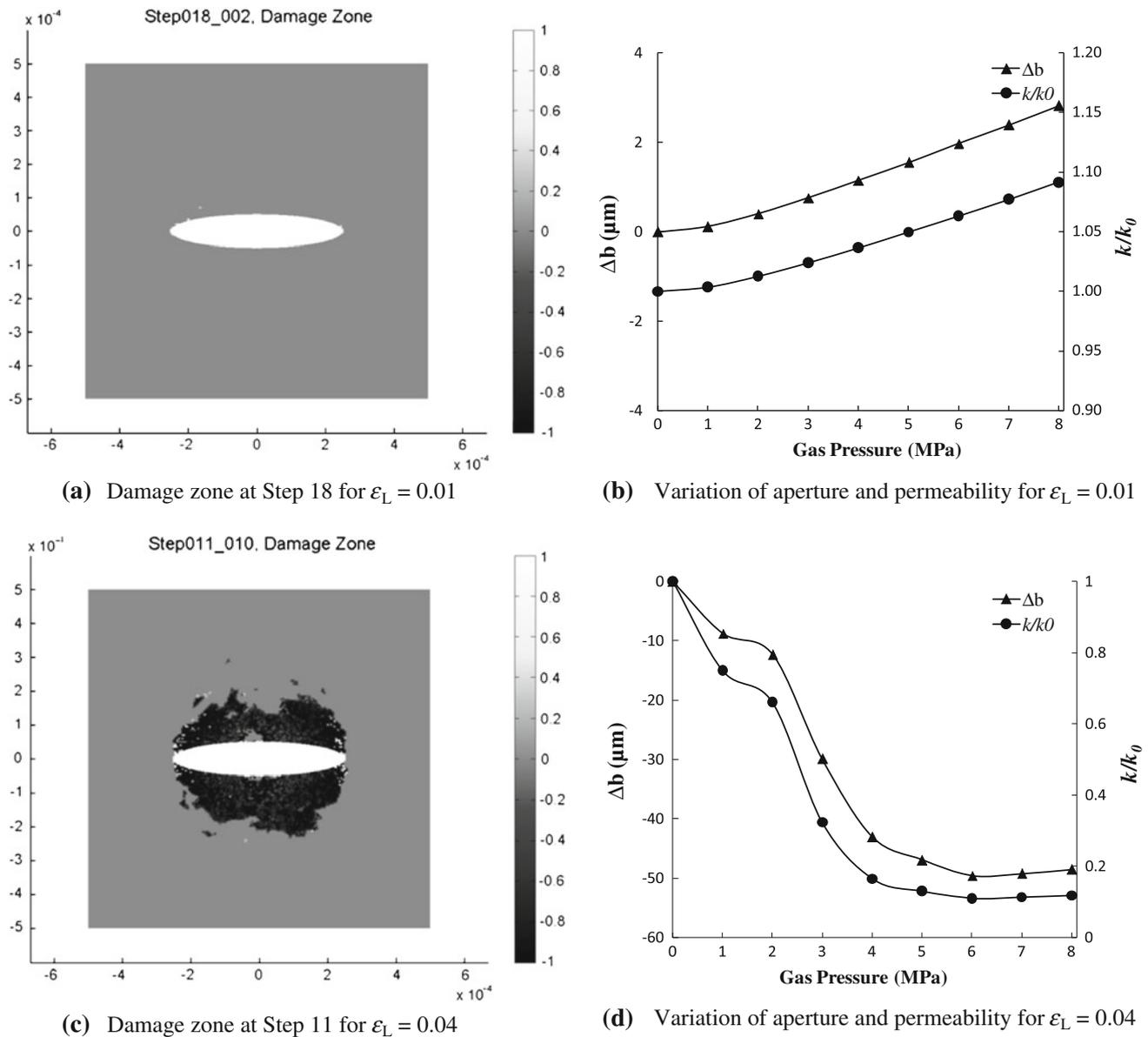
**Fig. 6** Numerical results for Scenario IV: **a** damage zone distribution and **b** variation of aperture and permeability for  $\varepsilon_L = 0.01$ ; **c** damage zone distribution and **d** variation of aperture and permeability for  $\varepsilon_L = 0.04$
