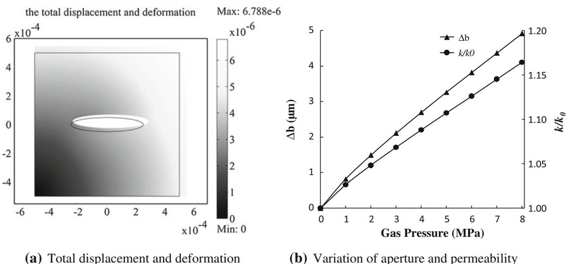
**Fig. 3** Numerical results for Scenario I: **a** total displacement and deformation, **b** variation of aperture and permeability with gas pressure
