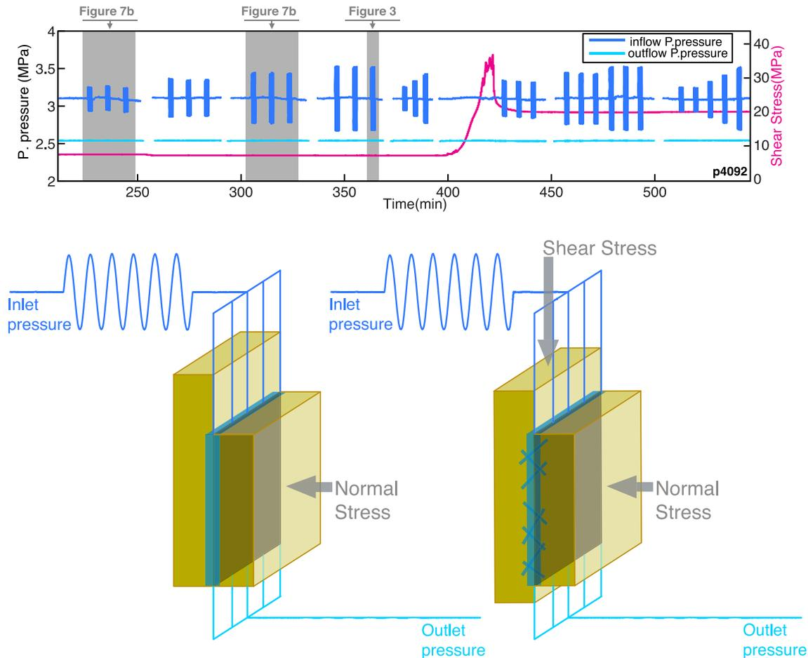
**Fig. 2.** Experiment overview. (Top) Experimental sequence consists of: (1) applying pore pressure oscillations at the inlet while holding constant the outlet pressure, (2) fracturing in-situ the sample, (3) resuming the dynamic stimulations. (Bottom) Geometry of the fluid flow for the intact and fractured sample. Once the sample fractured, the flow path is co-planar with the fracture plane.
