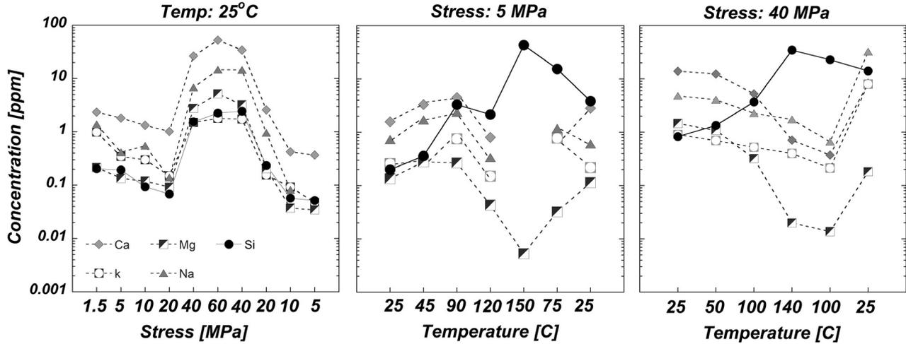
Fig. 3. Concentrations of the main elements (Al, Ca, K, Mg, Na, Si) as a function of the stress for the sample tested at room temperature (left panel) and as a function of the temperatures of the inlet fluid for the samples confined at 5 MPa (central panel) and 40 MPa (right panel). These values are also reported in Table 1 in the section: 'Test measurements'. Measurements below detection limits are omitted.
