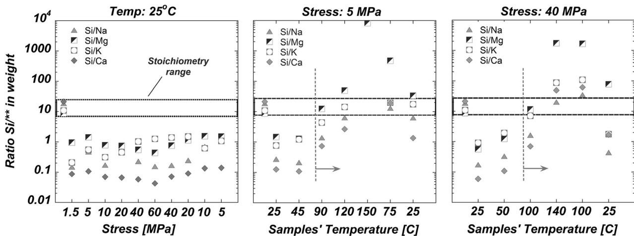
**Fig. 5.** Comparison between the theoretical/stoichiometric and the experimental weight ratios of the main elements with SiO<sub>2</sub> as a function of stress for the sample tested at room temperature (left panel) and as a function of the temperatures of the inlet fluid for the samples confined at 5 MPa (central panel) and 40 MPa (right panel). These values are also reported in Table 3 in the section: ‘*Test measurements*’.
