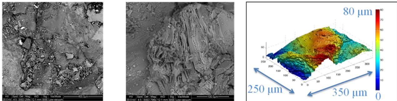
**Fig. 6.** Analysis using scanning electron microscopy including estimations of the roughness of the fractures via white light interferometry on surfaces of the following: (top) pristine sample of Westerly granite; (center) sample heated to 150°C confined at 5 MPa; and (bottom) sample heated to 140°C confined at 40 MPa.
