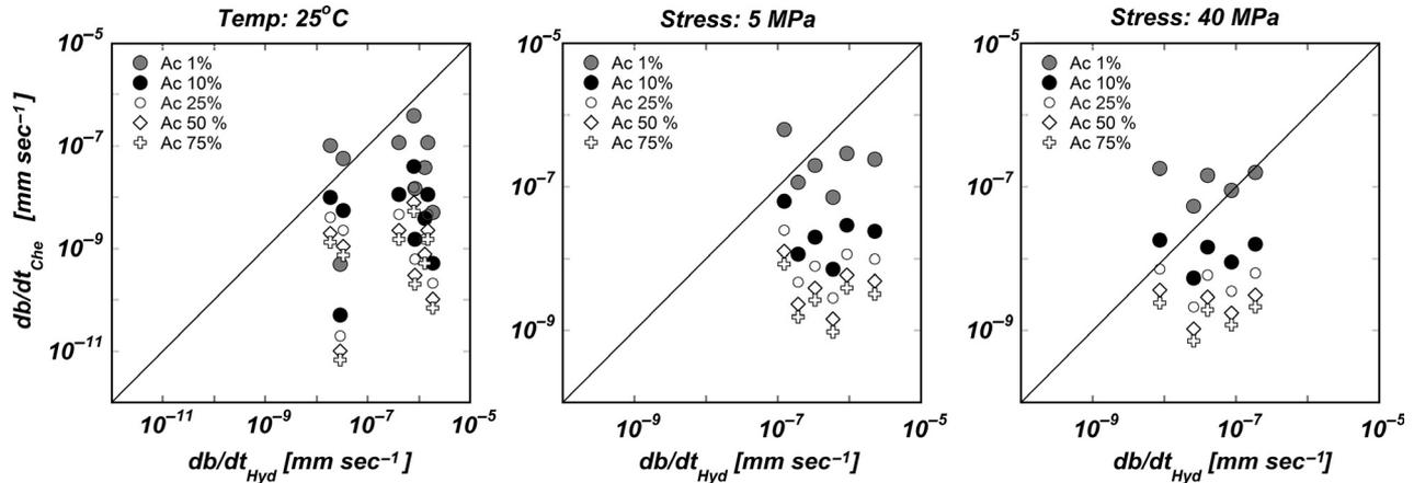
Fig. 4. Comparison between the rates of hydraulic aperture reduction  $db/dt_{Hyd}$  and the chemical rates of aperture reduction ( $db/dt_{Che}$ ).
