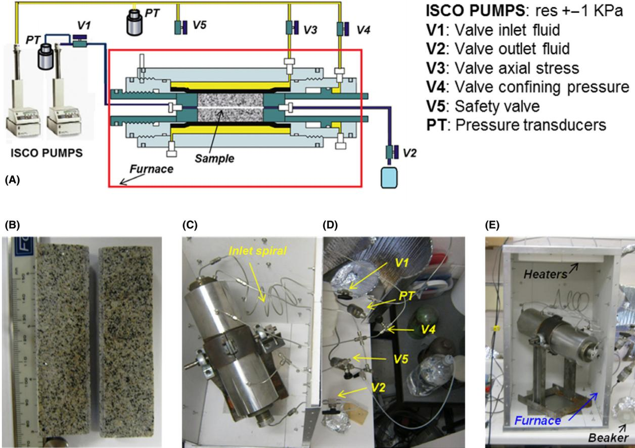
**Fig. 1.** Equipmental arrangement showing: (Top A) the schematic of the pressure vessel, the pressure intensifiers, the plumbing arrangement, and the furnace. In detail: the internal geometry of the pressure vessel with sample (shown in jacket) and the fluid access lines. (Bottom B): Westerly granite sample:  $\Phi$ : 25.4 mm and  $L$ :100 mm. (Bottom C and D): respectively, the plain and frontal views of the pressure vessel, the plumbing arrangement, and the furnace.
