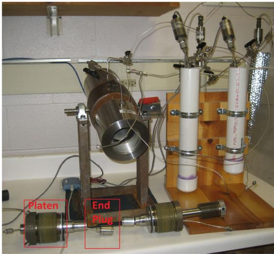
**Fig. 1** Hydraulic fracturing system. Containment vessel with platen and fluid feed assembly and cell end-caps in foreground
