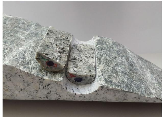
Fig. 1 Example of overcored specimen on top of one fracture surface
