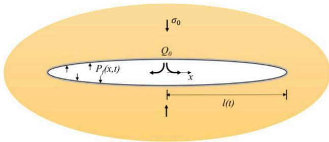
Fig. 2. Hydraulic fracture propagating in an impermeable elastic medium.
