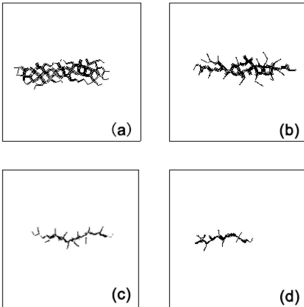
**Fig. 11.** Distribution of resulting hydraulic fractures in rock masses with randomly oriented joints under different in-situ stresses ( $t = 10$  s): (a)  $\sigma_y = 8$  MPa; (b)  $\sigma_y = 10$  MPa; (c)  $\sigma_y = 12$  MPa; (d)  $\sigma_y = 14$  MPa.
