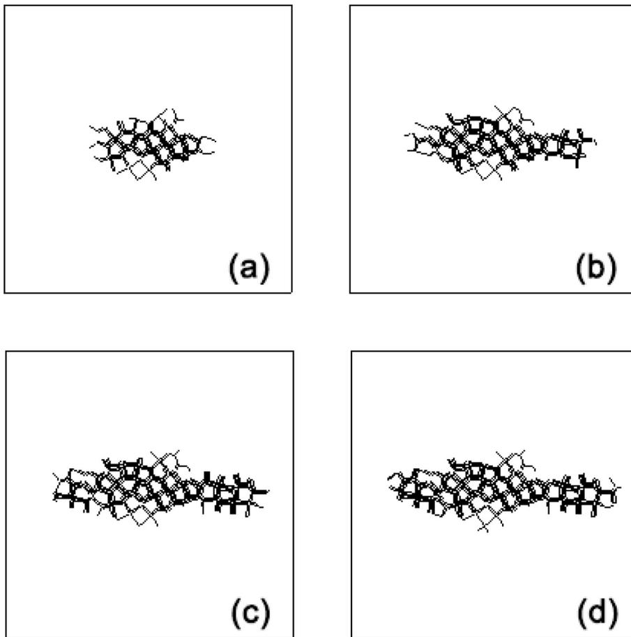
Fig. 12. Distribution of resulting hydraulic fractures in rock masses with random joints under different water injection rates ( $t = 10$  s): (a)  $Q_0 = 1 \times 10^{-4} \text{ m}^2/\text{s}$ ; (b)  $Q_0 = 2 \times 10^{-4} \text{ m}^2/\text{s}$ ; (c)  $Q_0 = 3 \times 10^{-4} \text{ m}^2/\text{s}$ ; (d)  $Q_0 = 4 \times 10^{-4} \text{ m}^2/\text{s}$ .
