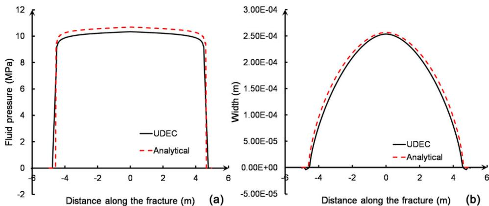
Fig. 5. (a) Pressure and (b) width distribution in the fracture after 10 s of injection.
