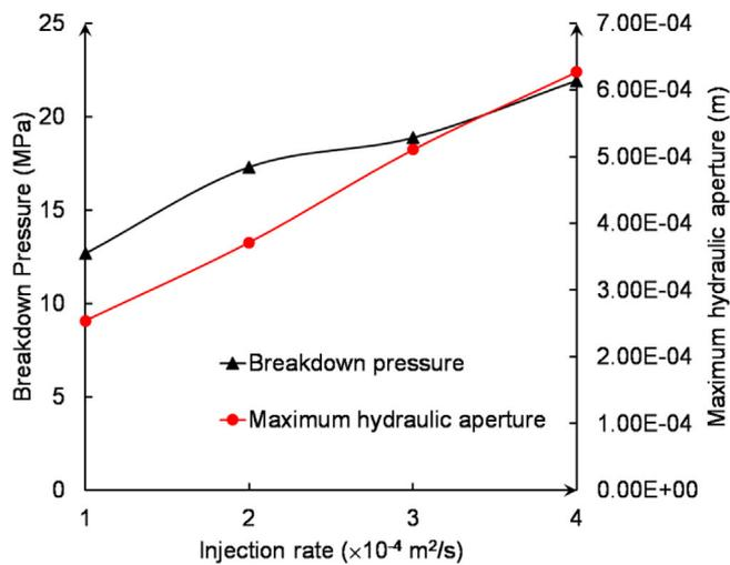
Fig. 13. The effect of water injection rate on breakdown pressure and maximum crack opening.
