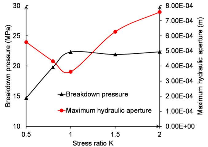
**Fig. 10.** Effect of stress ratio on breakdown pressure and maximum crack opening.
