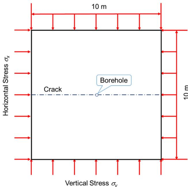
Fig. 3. Hydraulic fracturing in a model containing a prospective fracture at mid-height and with zero toughness.
