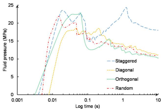
Fig. 8. Pore pressure with time for jointed rock masses: (a) diagonal; (b) staggered; (c) orthogonal; (d) random.
