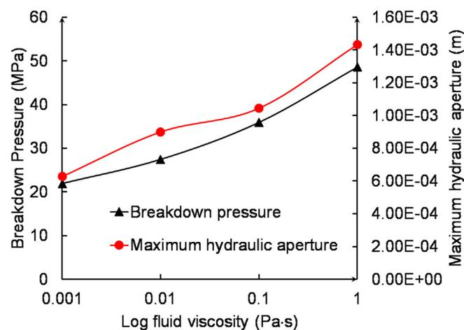
Fig. 15. The effect of fluid viscosity on breakdown pressure and maximum crack opening.
