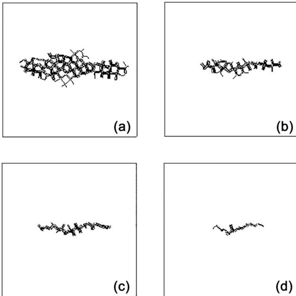
Fig. 14. Distribution of fractures in rock masses with random joints under different values of fluid viscosity ( $t = 10$  s): (a)  $\mu = 0.001$  Pa s; (b)  $\mu = 0.01$  Pa s; (c)  $\mu = 0.1$  Pa s; (d)  $\mu = 1$  Pa s.
