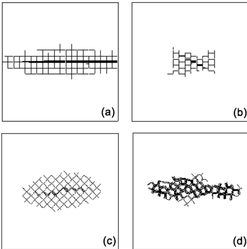
Fig. 7. Textures of fracture propagation in different jointed rock masses ( $t = 10s$ ): (a) orthogonal jointed rock mass; (b) staggered jointed rock; (c) diagonal jointed rock mass; (d) random jointed rock mass.
