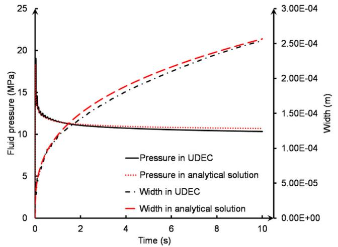
Fig. 4. Pressure and width at the well versus time for a KGD fracture of zero toughness.
