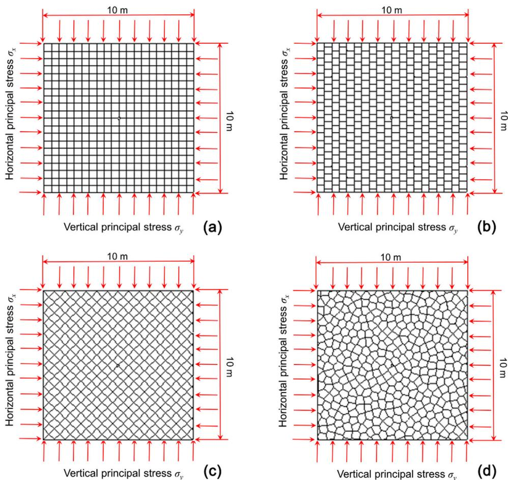
Fig. 6. Schematic diagram of HF model of rock masses: (a) orthogonal jointed rock mass; (b) staggered jointed rock mass; (c) diagonal jointed rock mass; (d) random jointed rock mass.
