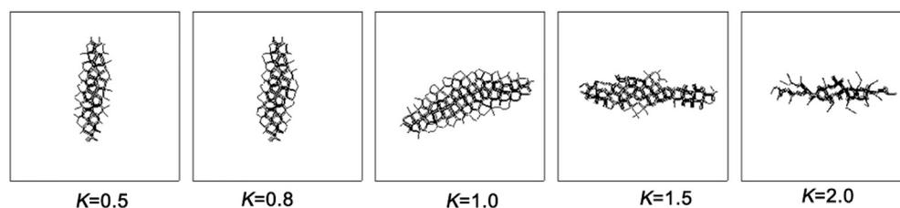
**Fig. 9.** Distribution of fractures in rock masses with randomly oriented joints under different stress ratio conditions ( $t = 10$  s).
