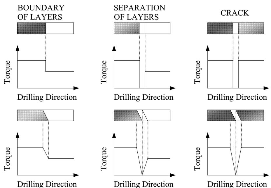
**Fig. 2** “Thrust valleys” associated with fractures in concrete block. (Reproduced with permission from Finfinger et al. 2000)
