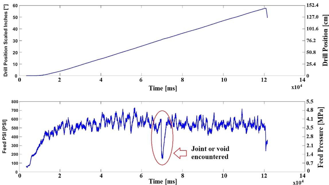
Fig. 5 Drill bit position and feed pressure (thrust) data
