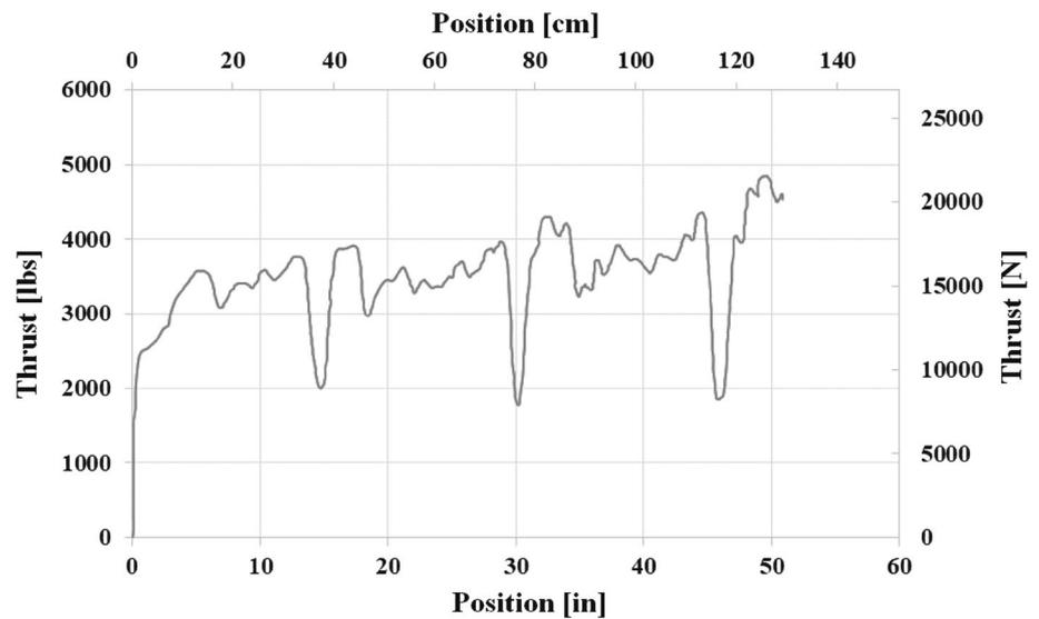
energy of drilling (SED) for identification of anomalies. The concept of SED was introduced by Teale at 1965 and could be calculated from drilling parameters. However, the WVU team noticed that SED showed significant variations in same rock material, and their research could not locate joints with the aperture less than 3.175 mm (0.125 in.) (Finfinger et al. 2000).
