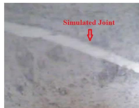
**c** A simulated joint in bore-scoping
