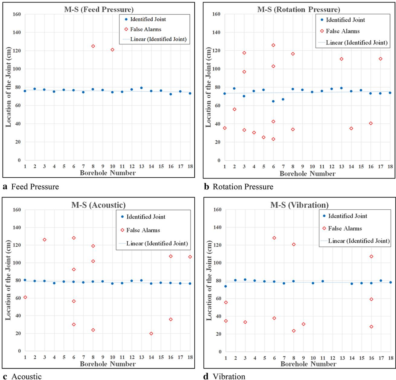
**Fig. 8** An example of joint detection results on the M–S composite sample by analyzing the feed pressure, rotation pressure, acoustic, and vibration data. **a** Feed pressure. **b** Rotation pressure. **c** Acoustic. **d** Vibration
