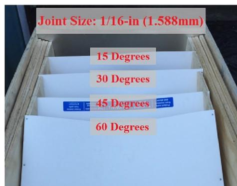
**b** Simulate inclined joints with Teflon material
