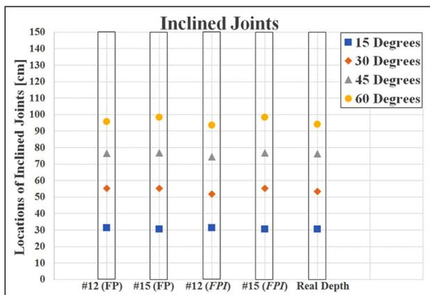
**Fig. 12** Joint detection results for drilling through inclined joints
