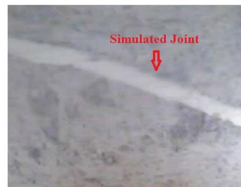
**c** A simulated joint in bore-scoping
