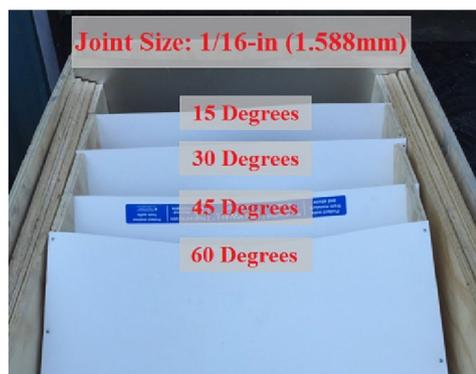
**b** Simulate inclined joints with Teflon material
