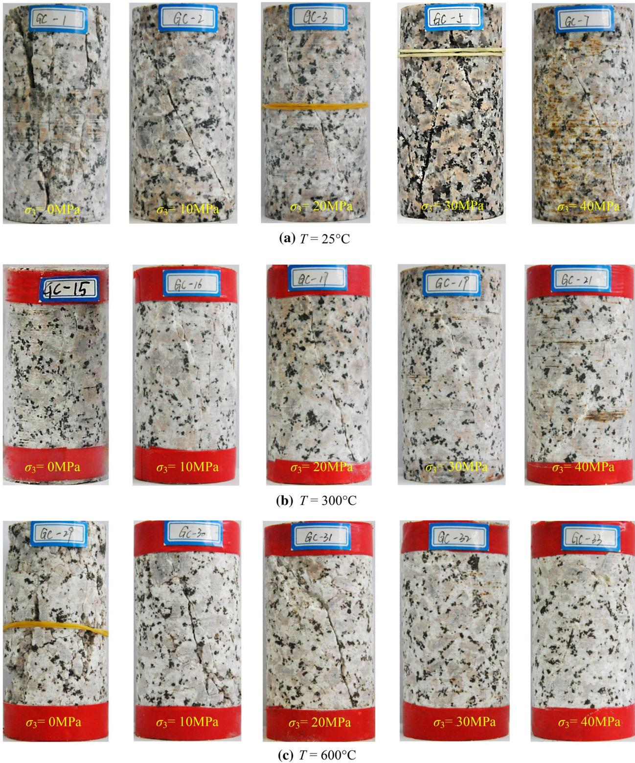
Fig. 18 Ultimate failure mode of granite specimen after high-temperature treatments under different confining pressures
