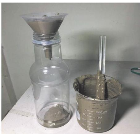
Figure 2. Testing device to define slurry flowability.
