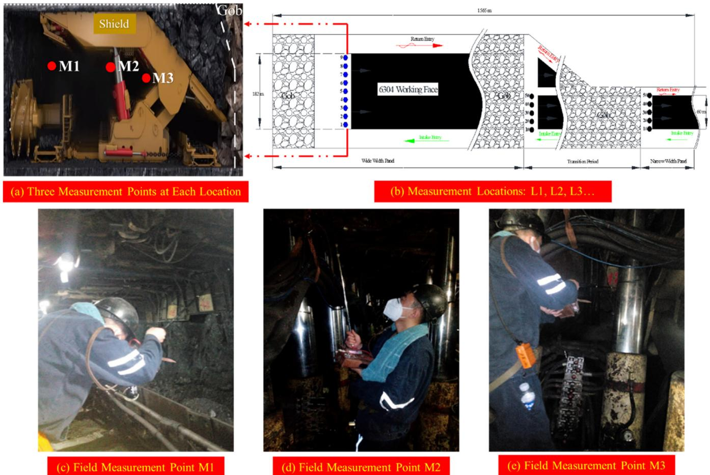
**Fig. 4.** Field investigation locations and measurement points at 6304 the longwall working face. (a) Three measurement points, M1, M2 and M3, are defined at each location. (b) Distributions of investigation locations at the 6304 working face. (c), (d), (e) Field investigator sampling.
