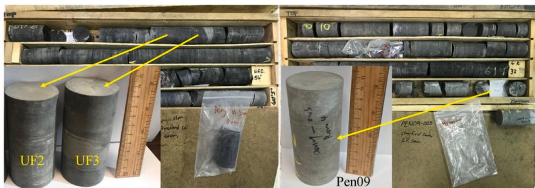
**Fig. 2.** Shale core specimens prepared for the fatigue test under uniaxial cyclic loading.
