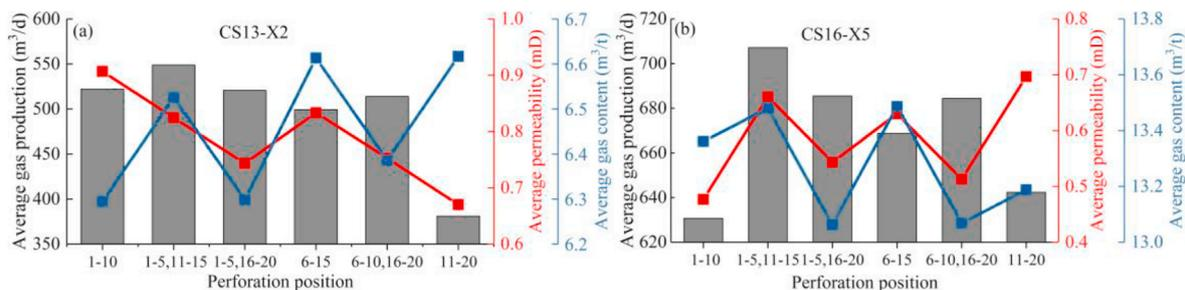
Fig. 17. Average gas production from different perforation configurations.
