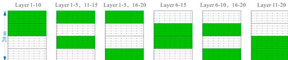
Fig. 15. Schematic diagram of the locations of perforations within SDUT CBM reservoirs.
