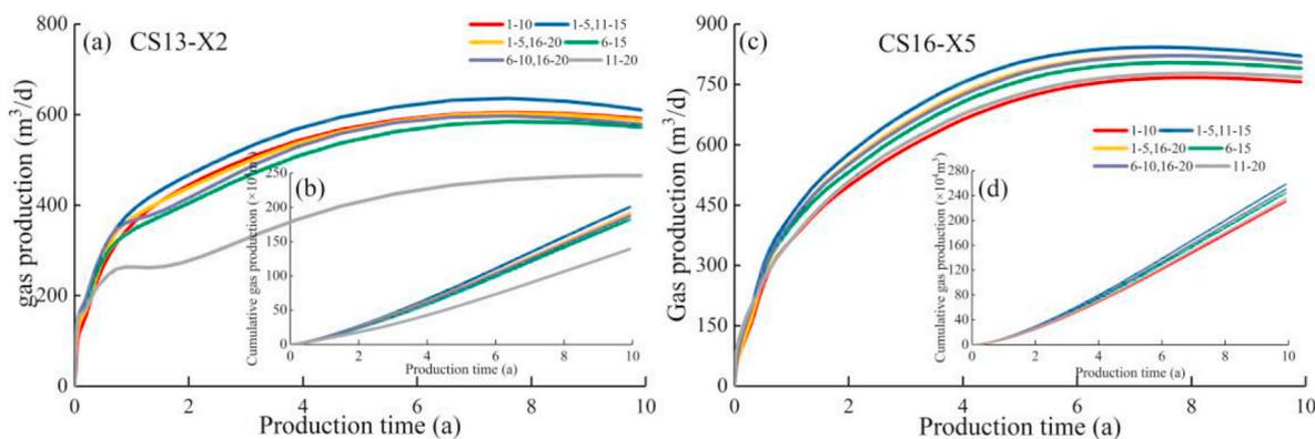
Fig. 16. Gas production rates for different combinations of perforation configuration.
