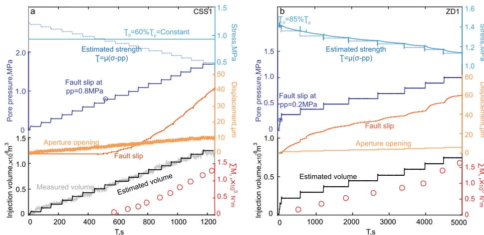
**Fig. 1** Typical observed fault displacement and cumulative moment over time as induced by fluid injection. The reactivated laboratory faults are under boundary conditions of (a) constant shear stress and (b) zero displacement. Measured variables and axes are color-coded to show the time evolution of fault fluid pressure, injection volume, fault slip and dilation, instantaneous strength, and cumulative moment magnitude.
