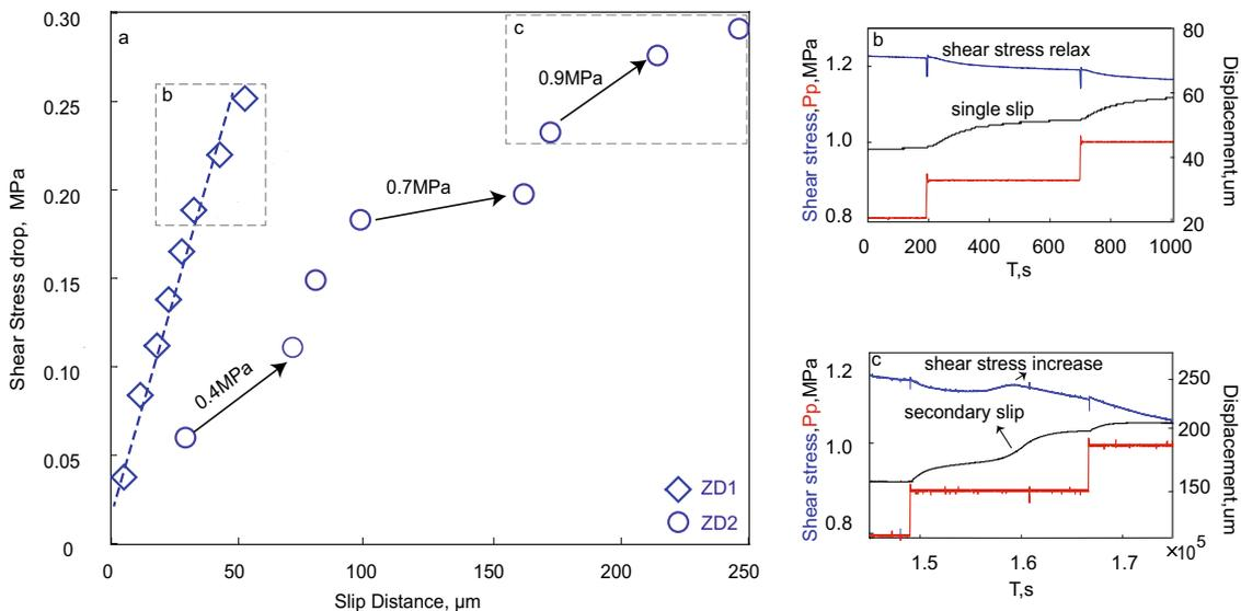
**Fig. 2 Shear stress drop/relaxation during fluid pressurization.** **a** Shear stress drop vs. slip displacement for tests ZD1 and ZD2. Experiment ZD1 shows a constant slope during fluid pressurization, while ZD2 features slope changes for the 0.4, 0.7, and 0.9 MPa pressurization steps. Pressurization step at 0.9 MPa for ZD1 (**b**) and ZD2 (**c**) are shown for comparison.
