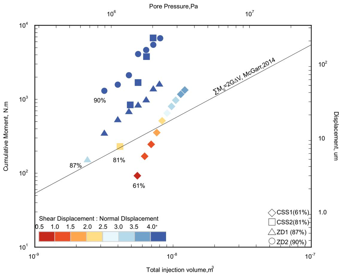
**Fig. 4 Cumulative moment magnitude versus total injection volume for all fluid pressurization steps in our experiments.** Symbol colors from hot to cold represent an increasing ratio of slip displacement to fault dilation. Specifically, in CSS1, the cumulative moment magnitude exceeds the classic limit when this ratio is  $>2$ . Initial stress ratios  $\tau/\tau_p$  are shown as percentages.
