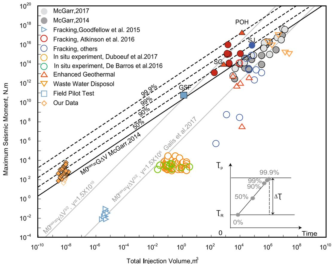
**Fig. 3 Maximum seismic moment versus total injection volume for fluid-injection-induced earthquakes.** Black line defines the upper limit of the seismic moment for assumed average stress. The black dashed lines represent solution with  $c$  values as shown in the lower-right inset. Gray solid lines represent maximum seismic moment and are added for completeness with two different  $\gamma$  values.
