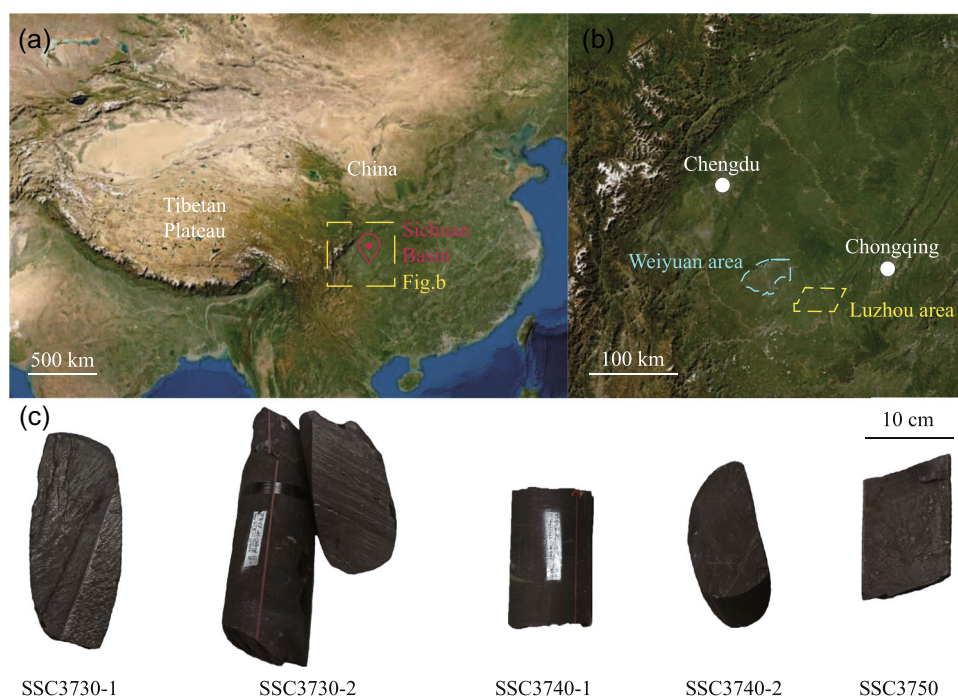
FIGURE 1 The location of the research region and the shale samples. (a) The research region of Sichuan Basin. (b) Luzhou area and Weiyuan area in the southeastern Sichuan Basin (Lei et al., 2020). (c) The sketch plots of the collected five shale samples.
