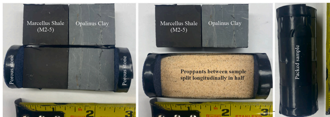
Fig. 5. The use of Opalinus clay to simulate and upscale the impact of slaking and particle ejection into the flowfield on the self-sealing behavior of fractures in Marcellus.
