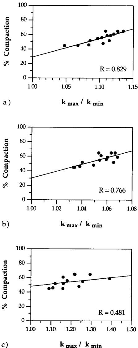
Fig. 8. Correlation between the degree of compaction and the degree of the magnetic fabric ( $k_{\max}/k_{\min}$ ) for (a) AMS fabric measured at room temperature, (b) AMS fabric measured at room temperature, (c) AMS fabric measured at low temperature, and (d) AARM fabric.
