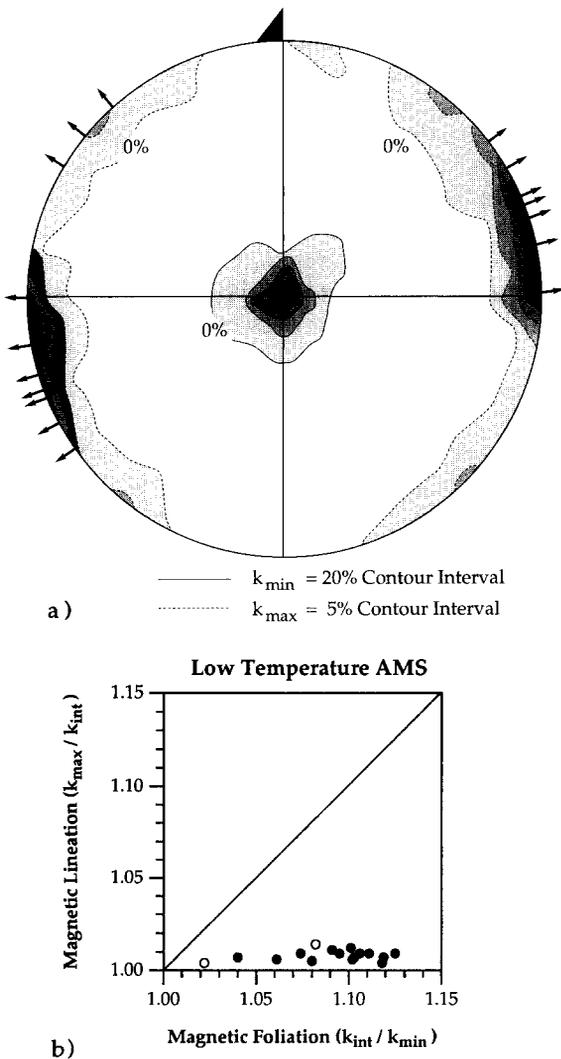
Fig. 5. (a) Density plot (equal-area, lower-hemisphere projections) of the  $k_{max}$  and  $k_{min}$  axes of the AMS magnitude ellipsoid measured at liquid nitrogen temperature. Arrows show the orientation of the long axes of chlorite grains. (b) Logarithmic plot of the principal axial ratios for the AMS at liquid nitrogen temperature.
