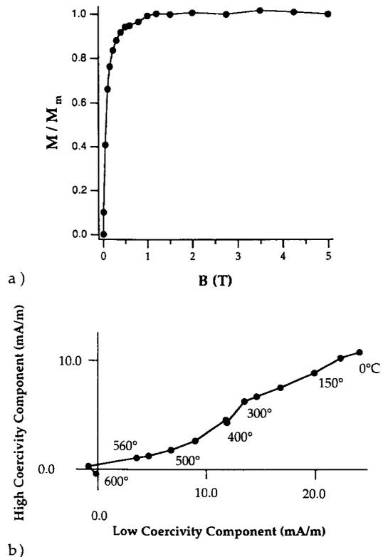
Fig. 6. (a) Acquisition of IRM for a black shale sample. (b) Vector diagram that shows the behaviour of the high- and low-coercivity component of the total IRM during thermal demagnetization.
