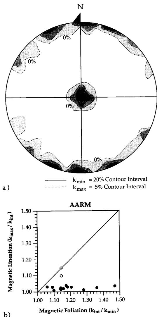
Fig. 7. (a) Density plot (equal-area, lower-hemisphere projections) of the  $k_{\max}$  and  $k_{\min}$  axes of the AARM magnitude ellipsoid. (b) Logarithmic plot of the principal axial ratios for the AARM.
