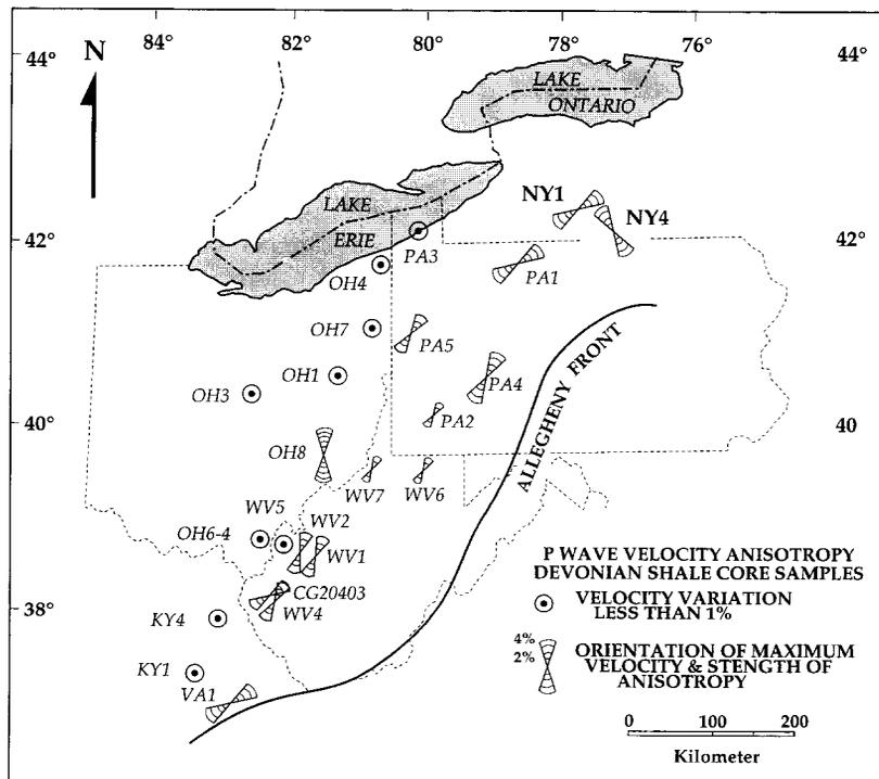
Fig. 1. Location map of drill cores that shows the magnitude and fast direction of the P-wave velocity anisotropy (after Evans et al., 1989a).
