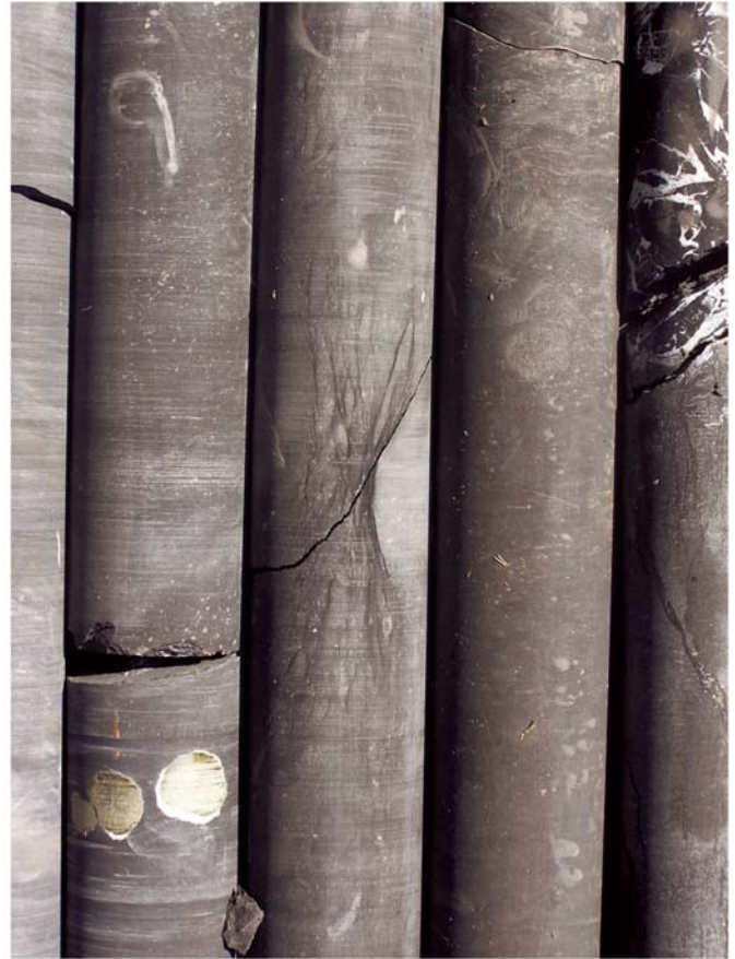
Figure 21. Core from the Purcell Member of the Marcellus showing a vertical extension of pyrite nodules, cleavage about a carbonate concretion, and calcite veins filling a cleavage duplex. This core comes from the Handiboe well located less than 2 km to the east of Stop 7.
