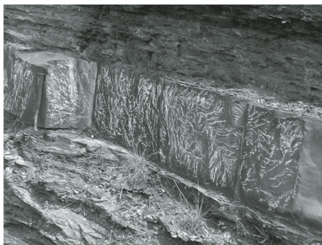
Figure 30. Joints in interbedded siltstone of the Brallier Formation in a road cut along Penn Street off Route 22 in Huntingdon, Pennsylvania (Ruf et al., 1998). Late-stage J_2 joints (chalk on two different joint surfaces with a hammer leaning against one of these) abutting a strike joint (joint propagating toward hammer).
