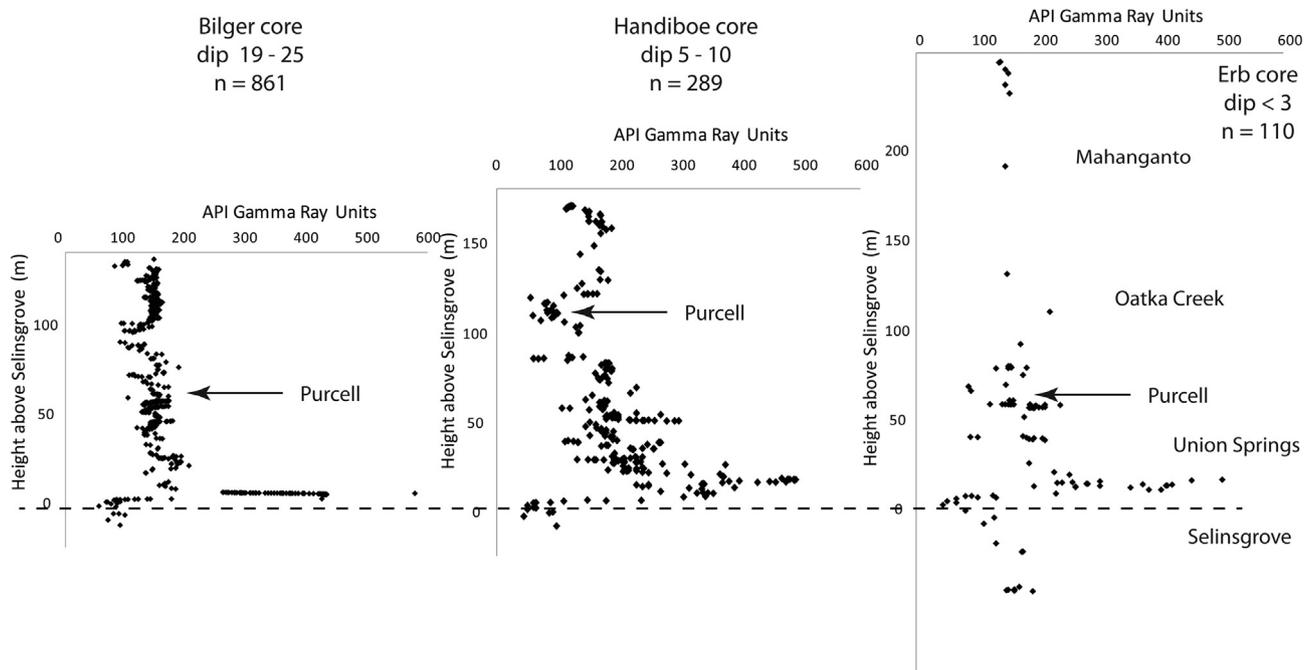
**Fig. 10.** API gamma ray units for rock matrix on which each slip surface sits. Note that one datum in the Bilger well approaches 600 API units. Number of slip surfaces in each well is indicated by *n*. Like Fig. 9, the height above the Selingsgrove is a vertical distance in a well bore. The horizontal datum is set at the Selingsgrove–Marcellus contact (dashed line).
