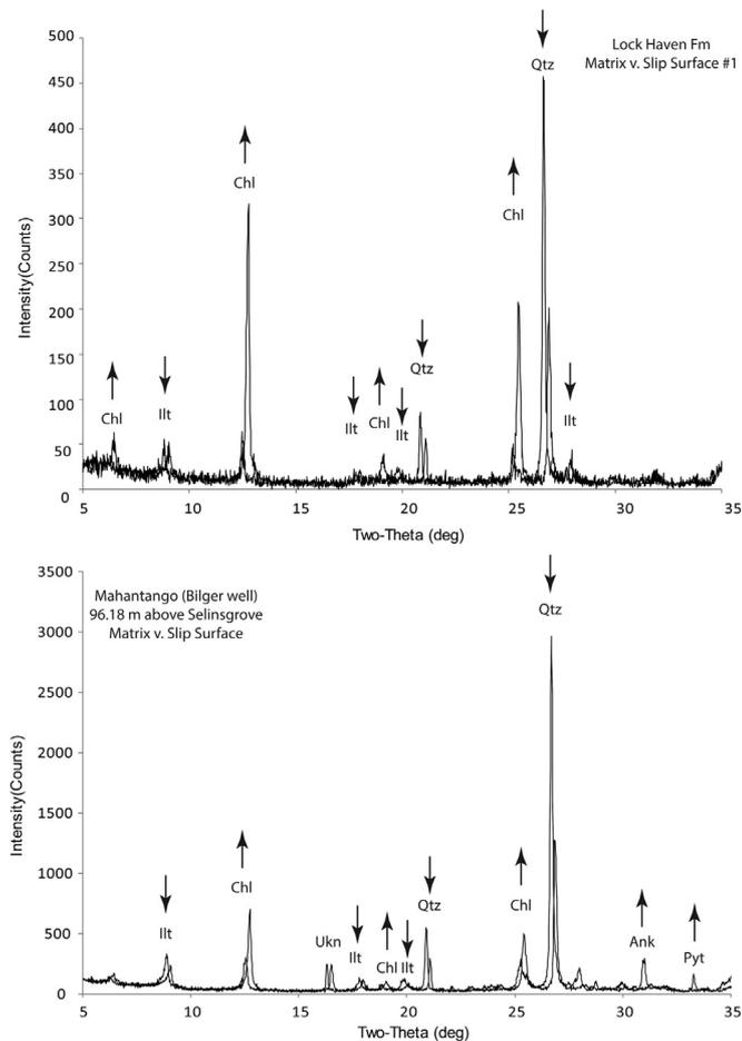
**Fig. 14.** XRD diffraction patterns from two slip surfaces in the Lock Haven Formation, Williamsport, PA and the Mahantango Formation, Bilger well. In each diagram the slip surface pattern is displaced to the right by  $0.2^\circ$  to allow for better comparison of the patterns. Arrows show which minerals increase and which decrease from the matrix to the slip surface. Qtz – quartz; Illt – illite; Chl – chlorite; Ank – Ankerite; Pyt – Pyrite; Unk – Unknown.
