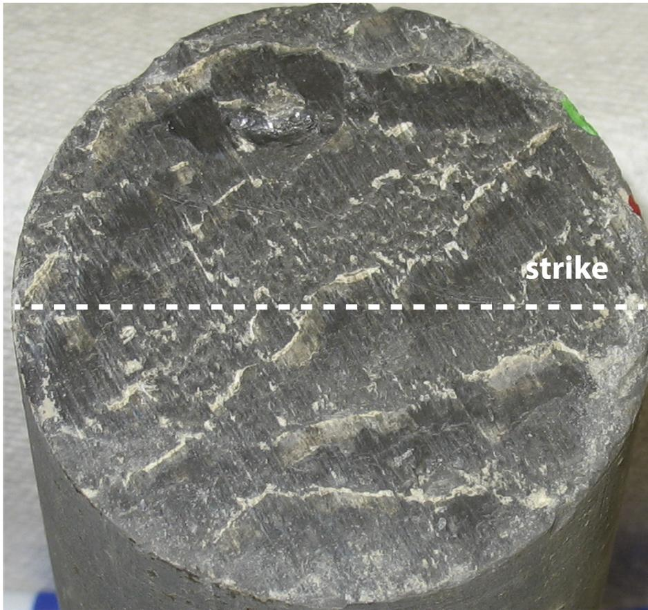
**Fig. 8.** Footwall sample of a slip surface showing fiber growth in the Mahantango Formation 122 m (by core) above the Selingsgrove Formation in the Bilger well. Core is oriented so that bedding strike is E–W and dip direction is toward the bottom of the photo. The angle between slip and dip is 30°.
