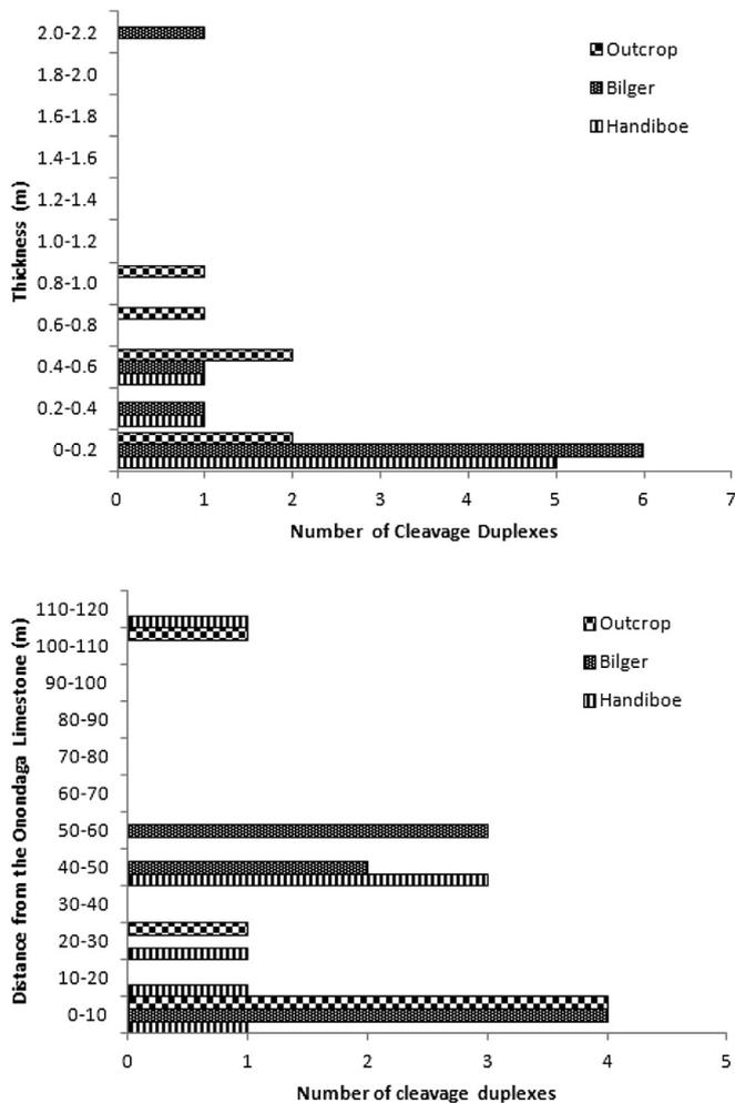
Fig. 7. For samples from both outcrop and core, the thickness of cleavage duplexes is binned in 20 cm intervals (top) and height of cleavage duplexes is binned in 10 m intervals above the Selinsgrove Limestone (bottom).
