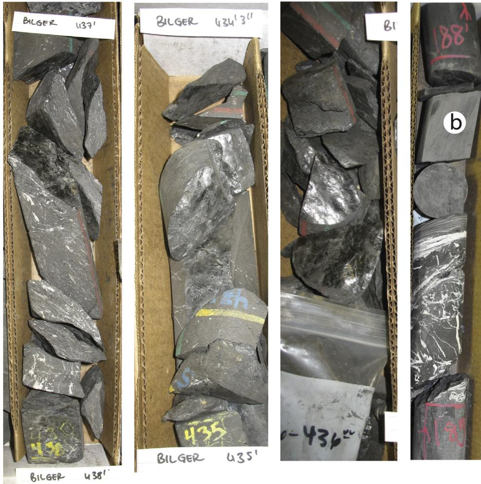
**Fig. 5.** Cleavage duplexes. (a) 53 cm thick cleavage duplex 2 m above the Selinsgrove Limestone in the Marcellus Formation at Newtown Hamilton showing a transport direction toward the foreland (left). (b) Cleavage duplexes in core: Bilger well (left three boxes) 2–6 m (by core) above the Selinsgrove Limestone; Handiboe well (right box) 112 m (by core) above the Selinsgrove Limestone.
