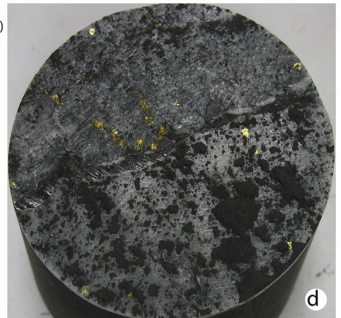
**Fig. 12.** Progressive mineral development on slip surfaces. (a) Pyrite and quartz entrained in fibers. (b) Pyrite entrained in a ridge-in-groove striations of chlorite. (c) Calcite and chlorite entrained in a mirror surface. (d) A matrix breccia entrained in calcite fibers.
