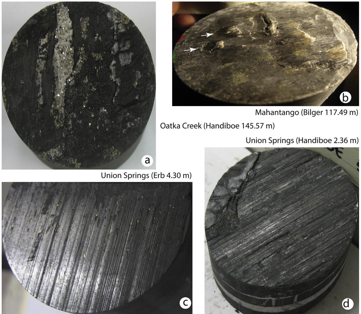
**Fig. 11.** The morphology of slip surfaces in the Mahantango-Marcellus section ranging from fibers (a and b) to ridge-in-groove striations (c and d).
