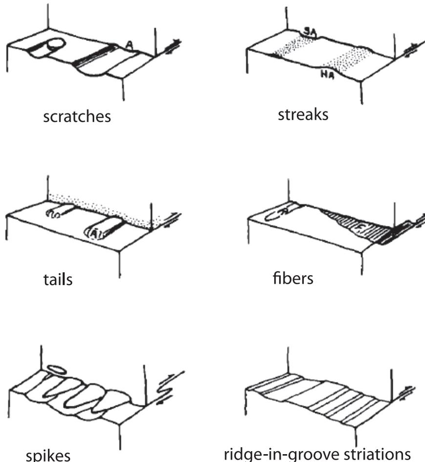
Fig. 2. Types of linear structures on slip surfaces (adapted from Means (1987)).
