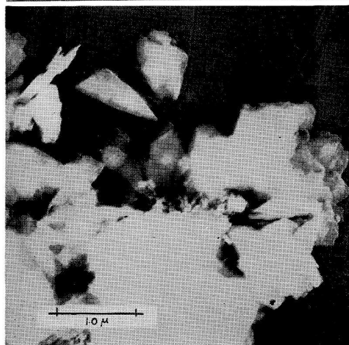
FIG. 1. Particles of calcined (1250°C) Resin "C" coke (above), and Texas coke (below). Both cokes were calcined prior to milling. Shadow-cast with chromium at 30° from horizontal.
