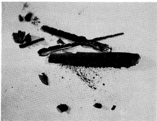
FIG. 6. D-type carbon deposited on A-type carbon plates.
