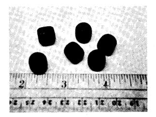
These sample pellets were taken from the finished lot of ten tons of pellets which were produced on schedule, met or exceeded all requirements, and provide a satisfactory replacement for the previously used  $\text{Sm}_20_3/\text{Al}_20_3$  material.
