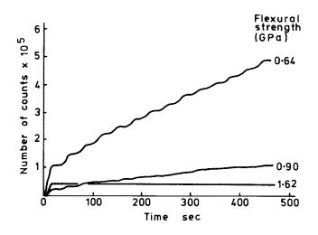
Figure 2 Acoustic emission from carbon-carbon composites during flexural cycling between 0 and 0.4~GPa
