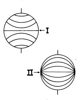
Figure 1. Mesophase Sphere Structures: (I) Standard Brooks-and-Taylor Structure, (II) Proposed Structure for Mesophase Spherules in Synthetic Model Pitches.
