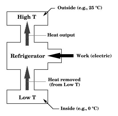
FIGURE 4-11. Schematic (thermodynamic) representation of a refrigerator.
