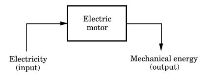
FIGURE 4-2. Energy conversion in an electric motor (electric-to-mechanical).
