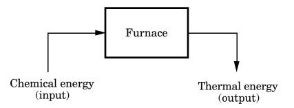
FIGURE 4-3. Energy conversion in a furnace (chemical-to-thermal).
