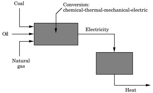
**FIGURE 4-13** Analysis of electric home heating using different primary energy sources.
