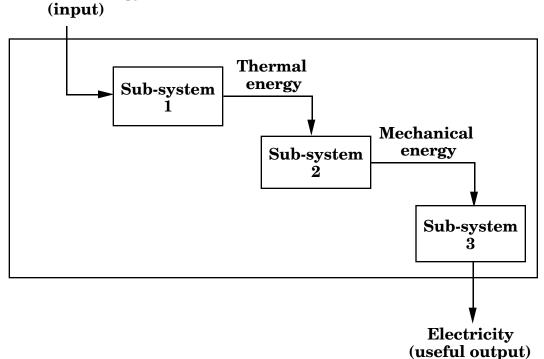
FIGURE 4-5. Energy conversion in an electric power plant.
