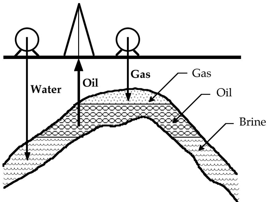
**FIGURE 8-9.** Enhanced oil recovery techniques: secondary recovery.
