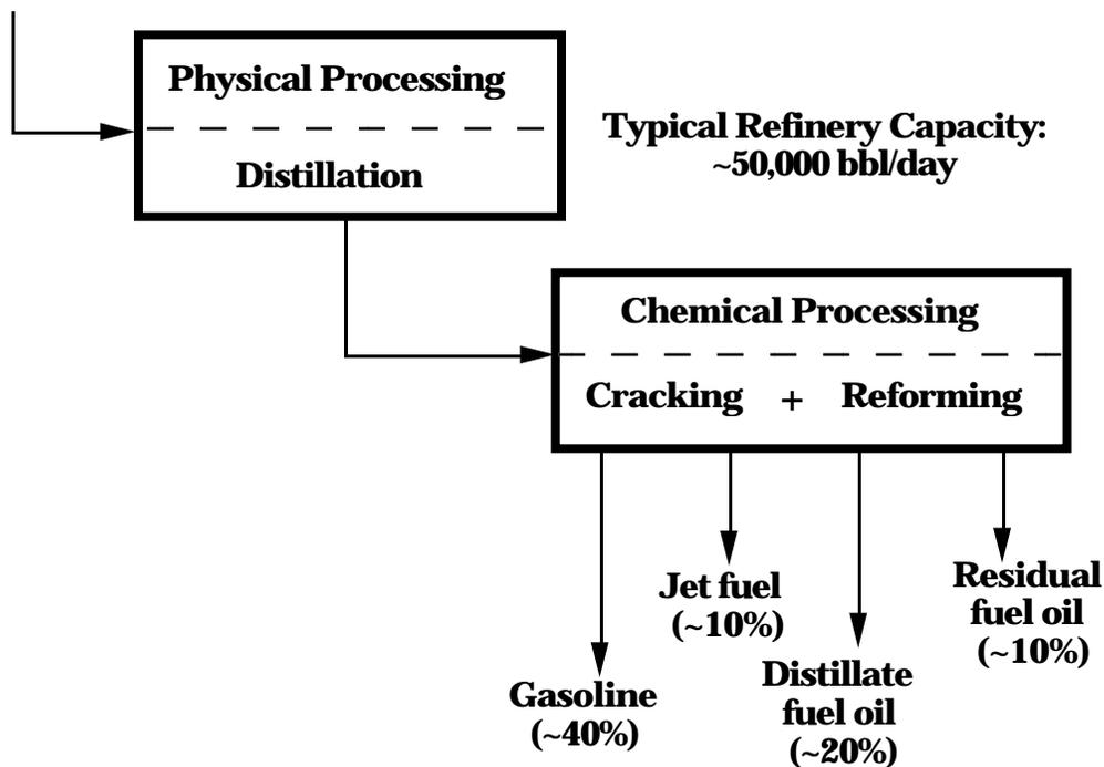
**FIGURE 8-12.** Schematic representation of a petroleum refinery.
