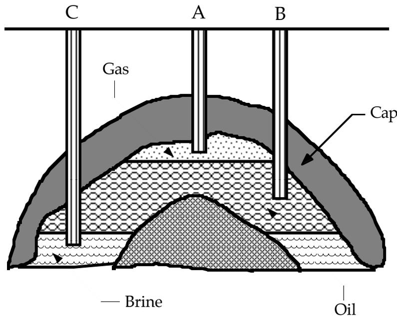
**FIGURE 8-7.** Selection of a site for petroleum drilling.
