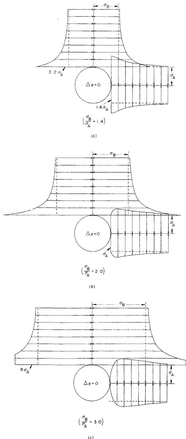
FIG. 14—STRESS STATES ABOUT A BOREHOLE FOR REGIONAL-STRESS RATIOS  $\sigma_B/\sigma_A$  OF 1.4, 2.0, AND 3.0.
