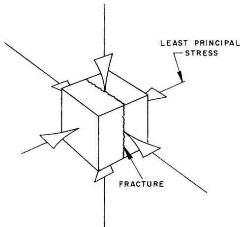
FIG. 1—STRESS ELEMENT AND PREFERRED PLANE OF FRACTURE.
