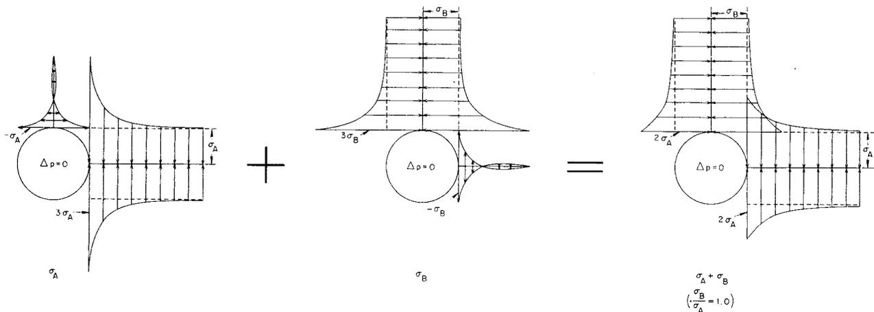
FIG. 13—SUPERPOSITION OF STRESS STATES ABOUT A WELLBORE DUE TO TWO HORIZONTAL PRINCIPAL STRESSES OF EQUAL MAGNITUDE.
