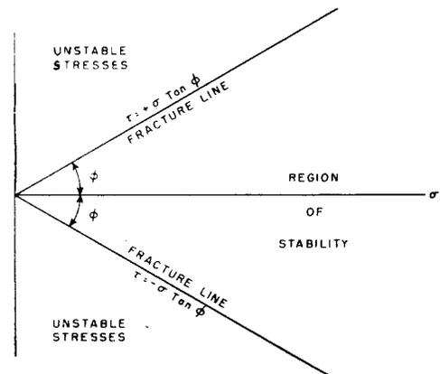
FIG. 8—MOHR ENVELOPES FOR SAND SHOWING CURVES OF VALUES OF  $\sigma$  AND  $\tau$  AT WHICH SLIPPAGE OCCURS.
