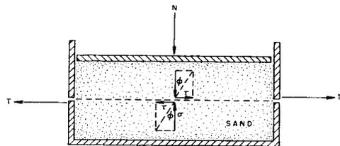
FIG. 7—SHEAR BOX FOR MEASURING RATIO  $\tau/\sigma$  AT WHICH SLIPPAGE OCCURS.
