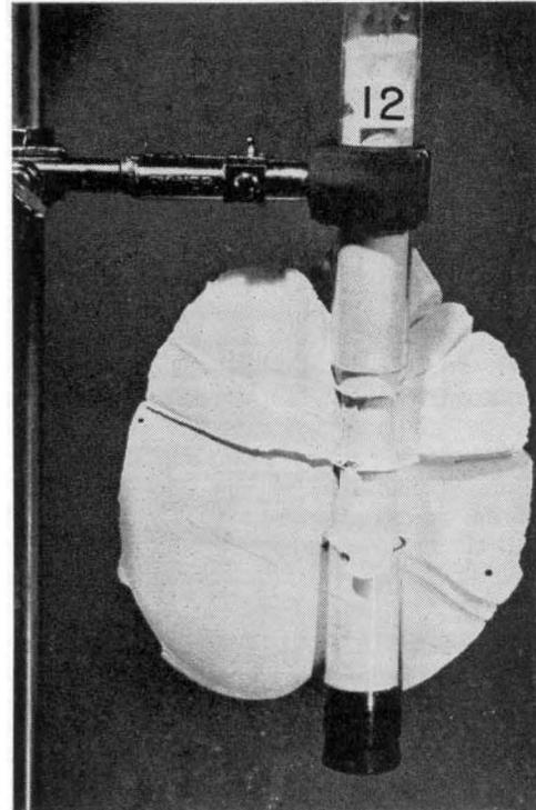
FIG. 23—VERTICAL FRACTURE PRODUCED UNDER STRESS CONDITIONS ILLUSTRATED IN FIG. 21.
