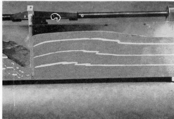
FIG. 3—SAND-BOX EXPERIMENT SHOWING THRUST FAULT.
