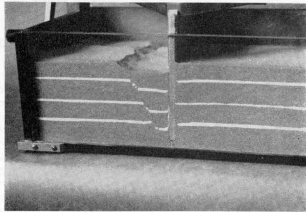
FIG. 2—SAND-BOX EXPERIMENT SHOWING NORMAL FAULT.
