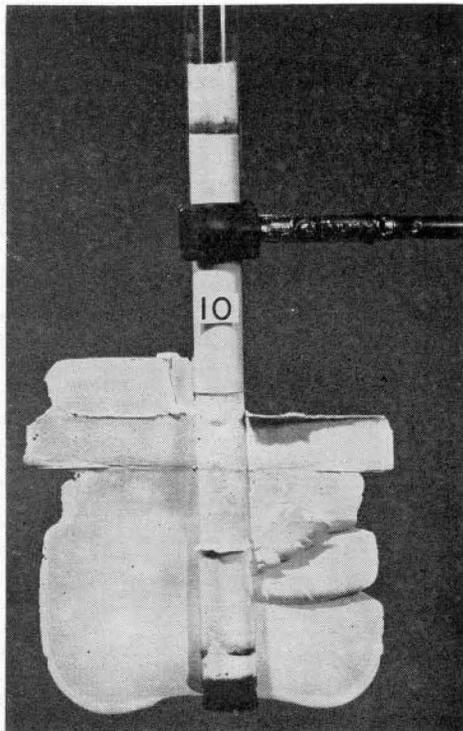
FIG. 25—VERTICAL FRACTURE IN STRATIFIED GELATIN.
