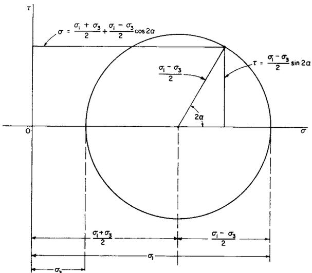
FIG. 6—MOHR DIAGRAM SHOWING NORMAL STRESS  $\sigma$  AND SHEAR STRESS  $\tau$  ON PLANE OF ORIENTATION  $\alpha$  IN TERMS OF  $\sigma_1, \sigma_3$ , AND  $\alpha$ .
