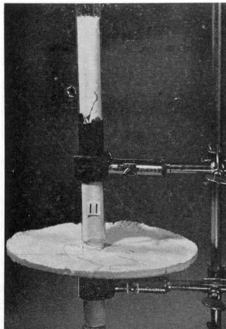
FIG. 26—HORIZONTAL FRACTURE IN STRATIFIED GELATIN.
