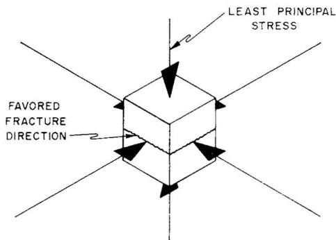
FIG. 22—EXPERIMENTAL ARRANGEMENT FOR PRODUCING THE LEAST STRESS IN A VERTICAL DIRECTION.
