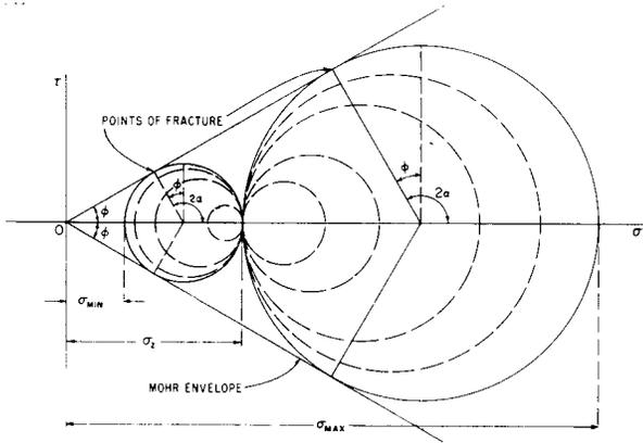
FIG. 9—MOHR DIAGRAM SHOWING THE POSSIBLE RANGE OF THE HORIZONTAL STRESS FOR A GIVEN VERTICAL STRESS  $\sigma_z$ . THE HORIZONTAL STRESS CAN HAVE ANY VALUE RANGING FROM APPROXIMATELY ONE-THIRD THE VERTICAL STRESS, CORRESPONDING TO NORMAL FAULTING, TO APPROXIMATELY THREE TIMES THE VERTICAL STRESS, CORRESPONDING TO REVERSE FAULTING.
