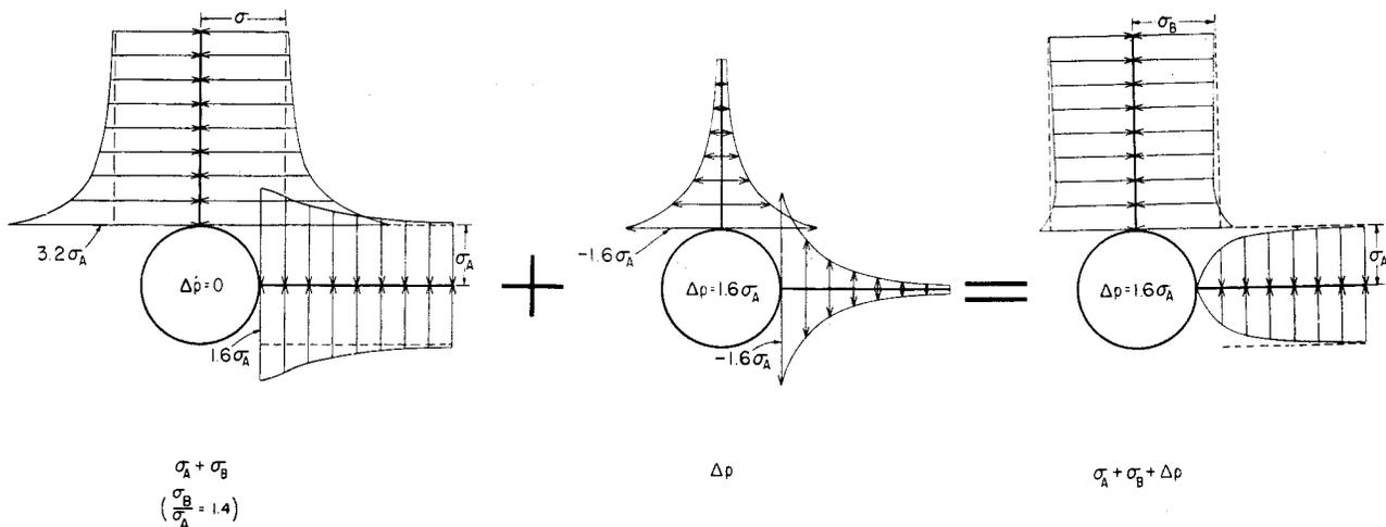
FIG. 16—SUPERPOSITION OF THE STRESSES DUE TO A PRESSURE  $\Delta p$  OF  $1.6 \sigma_A$  UPON THE STRESSES AROUND A WELLBORE WHEN  $\sigma_B/\sigma_A$  IS 1.4.
