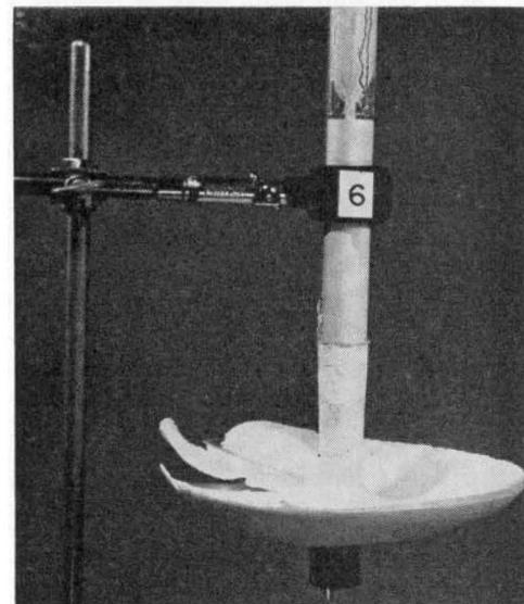
FIG. 24—HORIZONTAL FRACTURE PRODUCED UNDER STRESS CONDITIONS ILLUSTRATED IN FIG. 22.
