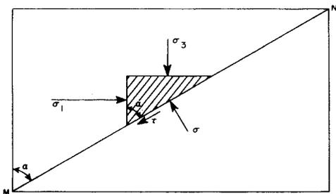
FIG. 5—STRESSES  $\sigma$  AND  $\tau$  ON PLANE OF ARBITRARY ANGLE  $\alpha$ .
