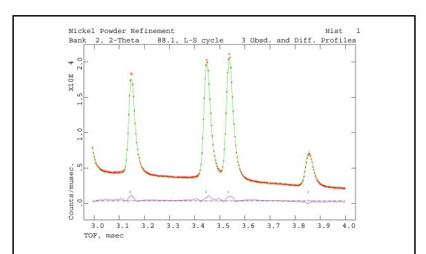
As you can see there is a fairly good match between  $I_0$  and  $I_c$ . The only difference here is a slight intensity mismatch for each reflection. Type ' $\downarrow$ ' if needed to continue; again you will have the option to view a portion of the initial plot range.
