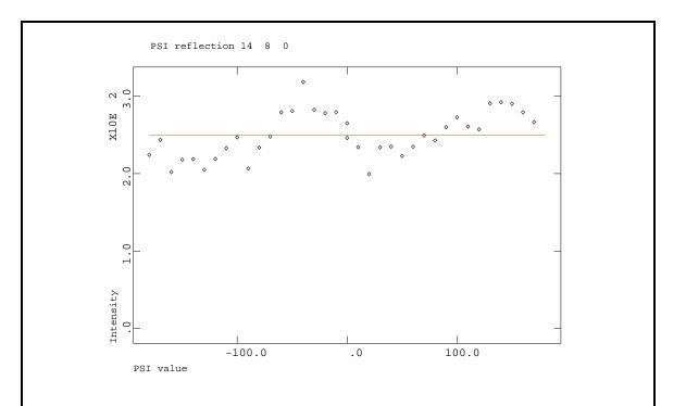
This  $\psi$ -scan shows the typical sinusoidal variation due to absorption from a non-spherical crystal. If there was more than one  $\psi$ -scan reflection set they would be plotted in turn. As for the other plots enter ' $\downarrow$ ' if necessary to get the next prompt.
