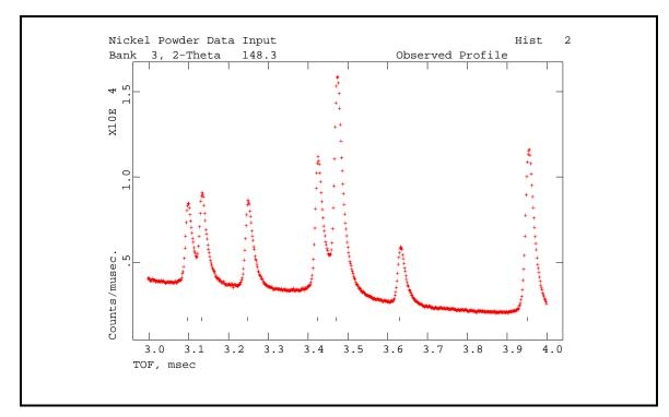
Again the blinking cursor indicates that the plot is finished. In this plot the marker positions are quite close to the peak center positions and are satisfactory. Type 'بل' if needed to continue.
