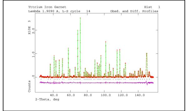
Clearly there are no longer any major differences between the observed and calculated profiles; the residuals are 3-5%. An exception is the large peak at  $\sim$ 150°; the remaining
