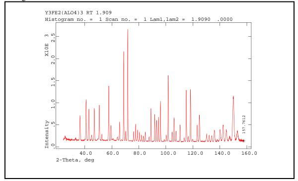
The minimum d-spacing sets the upper  $2\Theta$  limit for the calculations and is required before you can exit the histogram editing menu. The  $2\Theta$  value for end of the scan is noted in the above figure. It is probably easier to set it with the '**T**' option and give a maximum  $2\Theta$  of '**159**' that is just beyond the end of the data.
