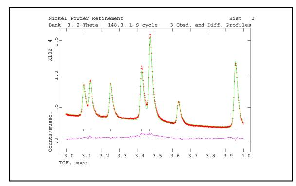
The major feature in this difference curve is a broad peak at  $\sim$ 3.45 msec; this is the (111) reflection offset by one TOF frame. Type ', ' if needed to continue.
