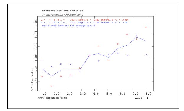
This plot shows the normalized intensities for both standards plotted as symbols along with their average as a solid line. Notice that in this case all three curves are similar so that an average correction is appropriate. On some terminals you need to enter ' $\downarrow$ ' to get the next prompt.
