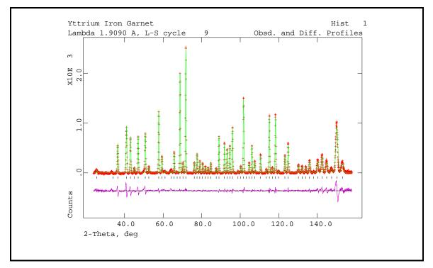
As you can see all the peak intensity errors have disappeared leaving only the peak shape errors at the ends of the pattern. Now refine the first four (U, V, W and asym) peak shape coefficients. You will also want to increase the number of background coefficients to six. Again run both **POWPREF** and **GENLES**. After this refinement has converged the profile should look like the next plot.
