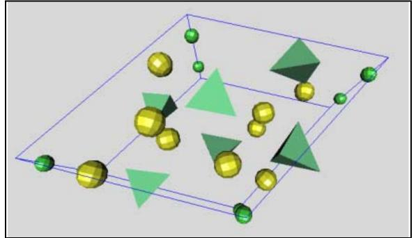
The Ca atoms are drawn in yellow, the F atoms in green and the  $PO_4^{3-}$  tetrahedra are also green; this color is associated with the P atom. The unit cell edges are also drawn. Notice that **VRSTPLOT** is still open, so that you can change the drawing interactively. A new
