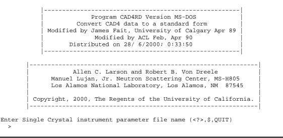
The file '/gsas/example/CAD4.PRM' is the instrument parameter file for the CAD4. It contains information that characterizes the Enraf-Nonius CAD4 diffractometer including attenuator data and the sense of rotation of the goniometer circles. Notice that the possibility of executing system commands is available here (the '\$' command).
