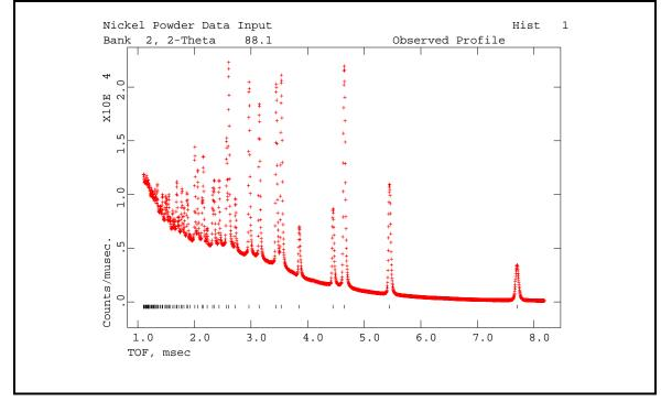
Notice that the reflection markers closely correspond to the peak positions. If the lattice parameters or diffractometer zero point had incorrect values the markers would not lie under the peak positions. This situation would probably cause **GENLES** to fail or at best converge very slowly. You would have to correct the values with **EXPEDT** and rerun **POWPREF** before continuing. You may have to type '-1' to continue; the following line will appear below the plot:
