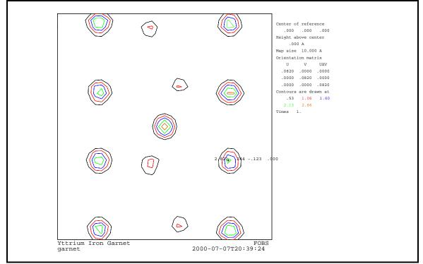
This is a  $10 \ge 10^{\text{Å}}$  ab-section centered at 0,0,0 looking down the *c*-axis of the garnet cell. The peak in the center is the first Fe/Al atom, the smaller peaks nearby are close to the O atom positions and the intermediate peaks to the right and left are Y atoms. A graphics cursor and a menu also appears on the plot. To move the cursor push the arrow keys (or
