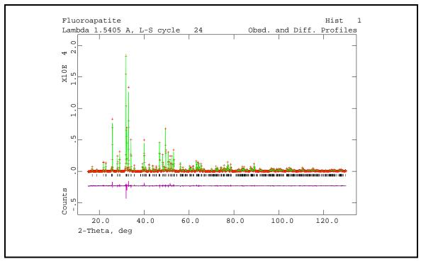
An expanded view of a selected high angle portion of the pattern shows how well the profile has been fitted.
