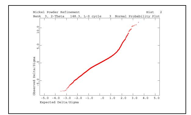
As you can see this plot gives a nearly straight line, excepting the extreme positive end, indicating that the  $I_0$ - $I_c$  values are for the most part normally distributed. The strong deviation at the high end is from the (111) reflection problem (see Section 4.3 of International Tables for Crystallography, Vol IV for a more complete discussion of normal probability plots). Type 'L' if needed to continue.
