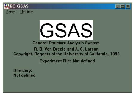
The message in the center of the screen results because **GSAS** fails to find an experiment file in your directory; the Unix version normally defines the first one alphabetically as the default experiment. Notice that the command line may also give the "node name" for the particular computer you are working on. For Unix systems, type **'help'** to display the main menu of components of **GSAS**.
