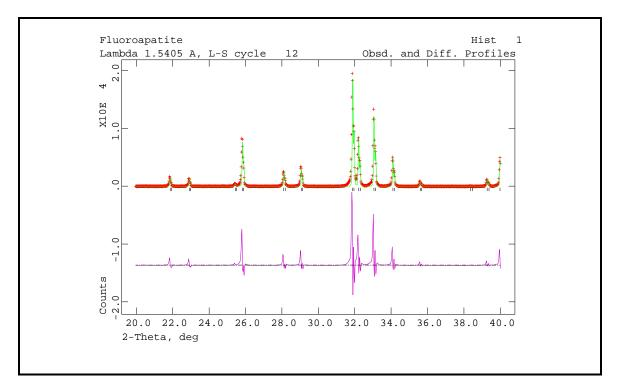
The fit is still quite poor but it is much better that before. The major problem now seems to be that the calculated profiles are not wide enough and that there is still some peak displacement error. The appropriate profile coefficients to vary are the Lorentzian coefficients 'LX' (particle size), 'LY' (microstrain) and 'shft' (sample displacement). Then run **POWPREF** and **GENLES**. The last cycle of least squares shows marked improvement.
