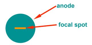
Filament geometry & electron focusing determine size, shape of focal spot, which influences size, shape of beam from tube
