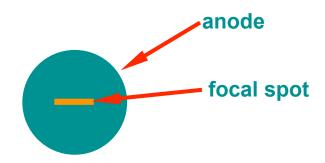
1st problem - tubes usually have liner focal spot w/ finite width microfocus tubes
