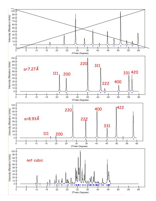
4. Derive the extinction rule for C-centering by calculating which (hkl)s systematically have F = 0. Follow the procedure discussed for I-
