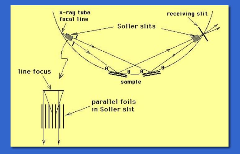
To maintain the focusing geometry, when counter is rotated at rate of  $2\theta$ /min, specimen is also rotated at rate of  $\theta$ /min
