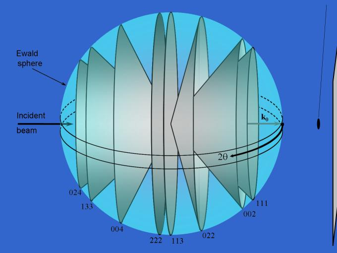
film, image plate, or area detector X-ray diffraction
